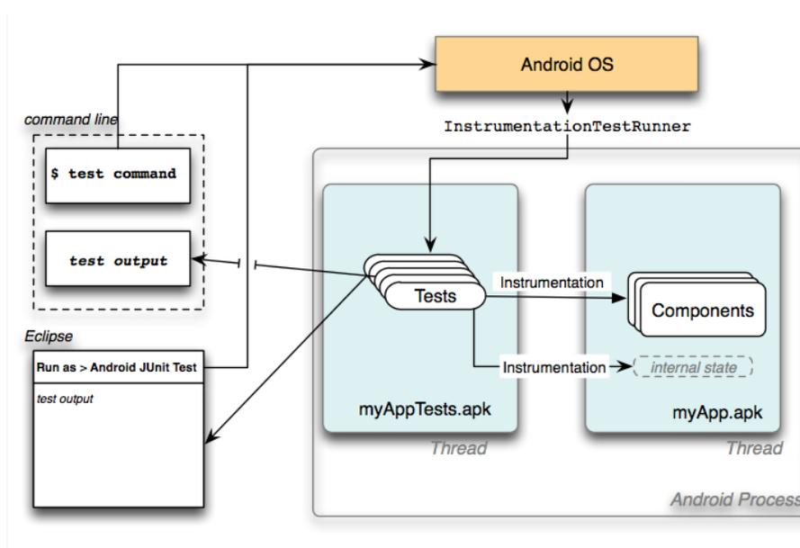
Figure 6.3: Instrumentation framework structure with its different components on- and off-site the device. From [22, Testing and Instrumentation].
