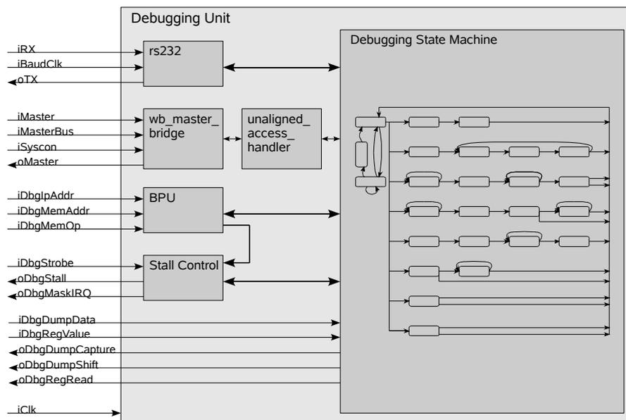
Figure 4.1: Overview of the newly implemented debugging unit
