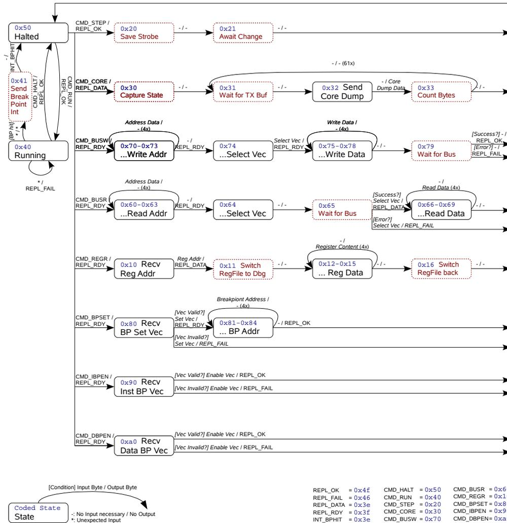
Figure 4.2: The extended FSM of the debugging unit, which is implemented in Verilog
