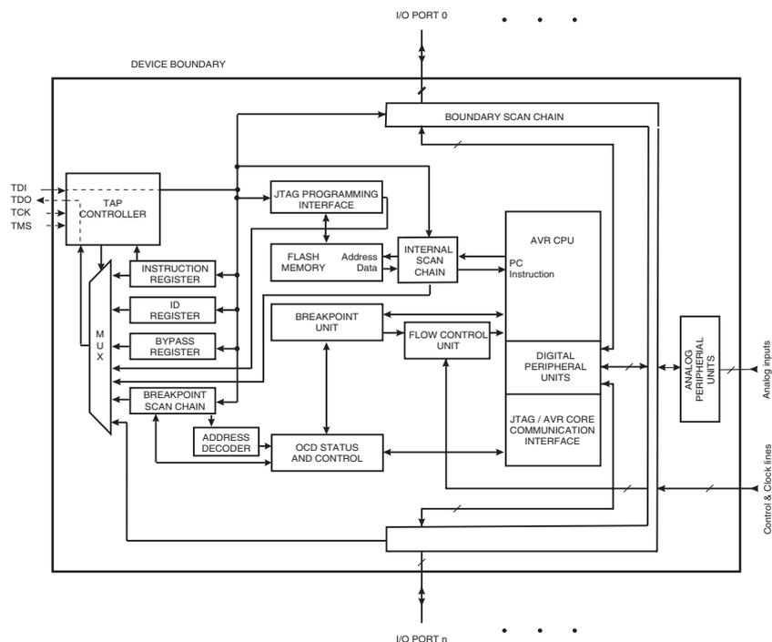
Figure 2.4: Block diagram of the *JTAG* test access port on the megaAVR [1]
