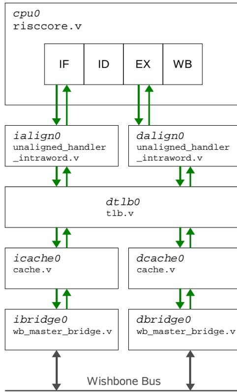
Figure 2.2: Standard memory access chain of the OpenProcessor
