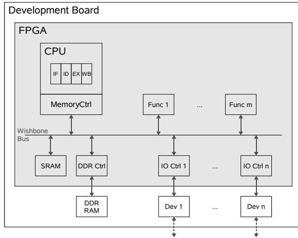
Figure 2.1: Logical view of the OpenProcessor Platform
