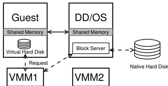
Figure 3.3: DD/OS - Client Architecture
