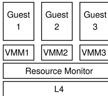
Figure 3.1: Virtualization Architecture
