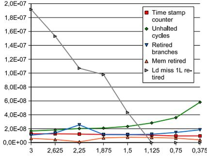
**Figure 4:** Weights of events for all clock gating speeds in J
