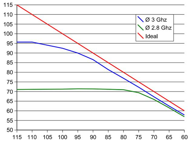
**Figure 8:** Average power usage for both frequency scaling settings. X-Axis is the maximum allowed power usage (W). Y-Axis is the actually used power. (W)
