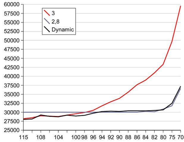
**Figure 9:** Average time in ms of the benchmarks for different values of maximum power. The first two and the last 3 X-Axis Sections have a distance of five. The rest have a distance of two.
