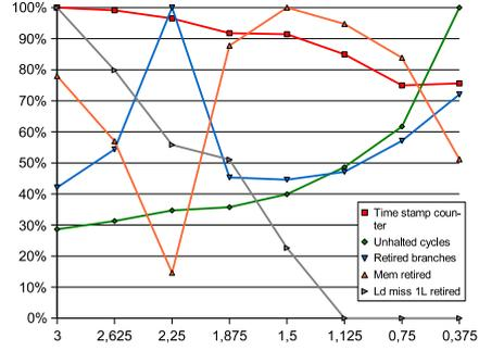
**Figure 5:** Weights of events for all clock gating speeds (relative)
