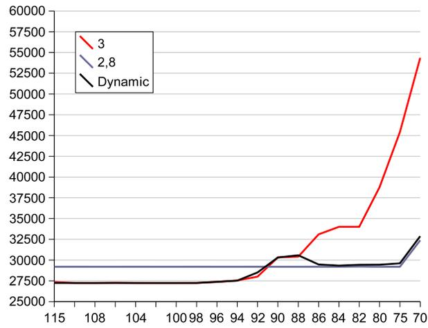
**Figure 10:** Used time in ms of *bench<sub>1</sub>* the benchmarks for different values of maximum power. The first two and the last three X-Axis Sections have a distance of five. The rest have a distance of two.
