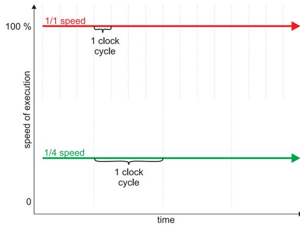
**Figure 2:** CPU state while frequency scaling
