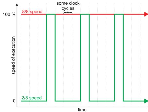
Figure 1: CPU state while clock gating
