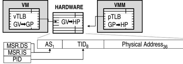
**Figure 4. Merging two levels of virtualized address translation into a single-level hardware TLB.**
