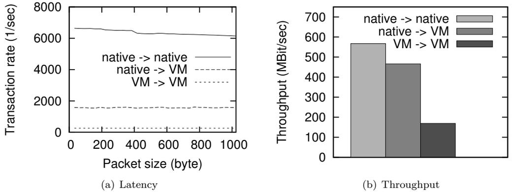
**Figure 8. Performance of Torus-Routed Virtualized Ethernet Networks.**
