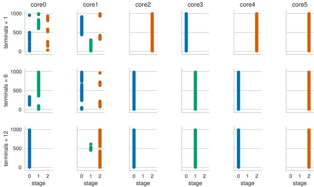
(b) Core Assignment over time (time on y-axis). The minimal transition algorithm leads to stable allocations, in particular for higher core counts.
