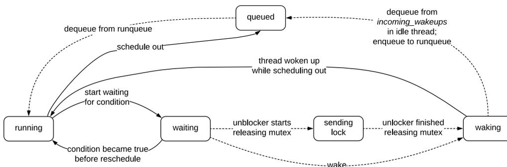
Figure 4.4: Upstream OSv wake-up-related thread state transitions: States *waiting*, *sending\_lock* and *waking* are ambiguous with regard to whether the thread is still scheduling out whether it has fully stopped executing. Dashed lines represent events asynchronous to thread execution, solid lines represent synchronous events.
