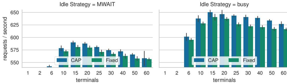
(a) TPC-C throughput. The y-axis is off-set. Error bars represent standard deviation.
