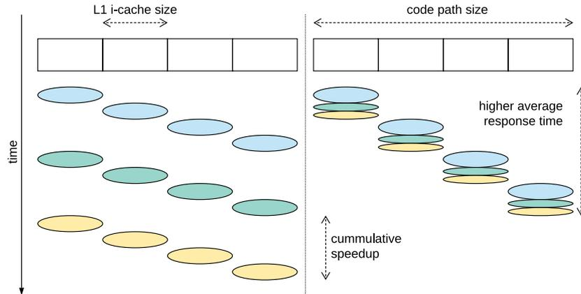
Figure 2.1: Idealized scenario of three threads (different colors) executing the same code path that does not fit into the L1 cache. **Left:** Each thread passes through the code completely before yielding CPU to the next thread. **Right:** A team of threads trickles down the code path in code segments that do not exceed the L1 i-cache size.
