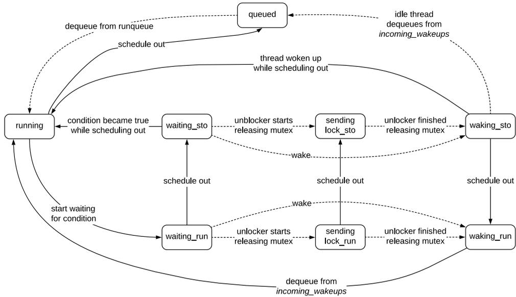
Figure 4.5: Modified OSv wake-up-related thread state transitions: All states are unambiguous about whether the thread is still running or completed scheduling out. Dashed lines represent events asynchronous to thread execution, solid lines represent synchronous events.
