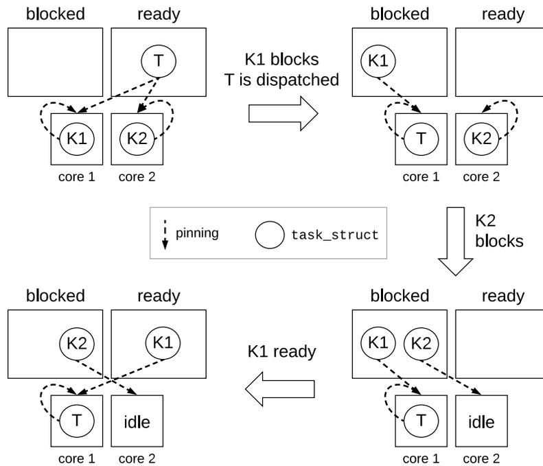
Figure 3.1: The proof-of-concept implementation is not work-conserving. When K1 becomes ready it should be dispatched to C2 immediately. But K1 is pinned to C1 due to the implementation of thread migration.
