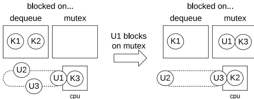
Figure 2.2: When a ULT issues a blocking syscall, the current KLT blocks. Another KLT must take over executing ULTs from the core's queue. Note that although there is a KLT for each ULT, the relationship is not fixed.
