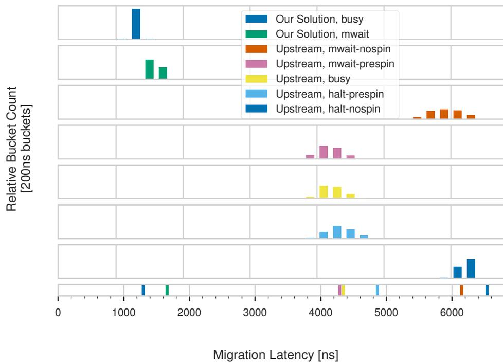
Figure 5.5: Histogram of `hopper` migration latencies with 200ns buckets, bars drawn at the center of each bucket. The last row shows the exact mean values. Our solution shows more than 70% lower migration latency and is less affected by `MWAIT` than upstream.
