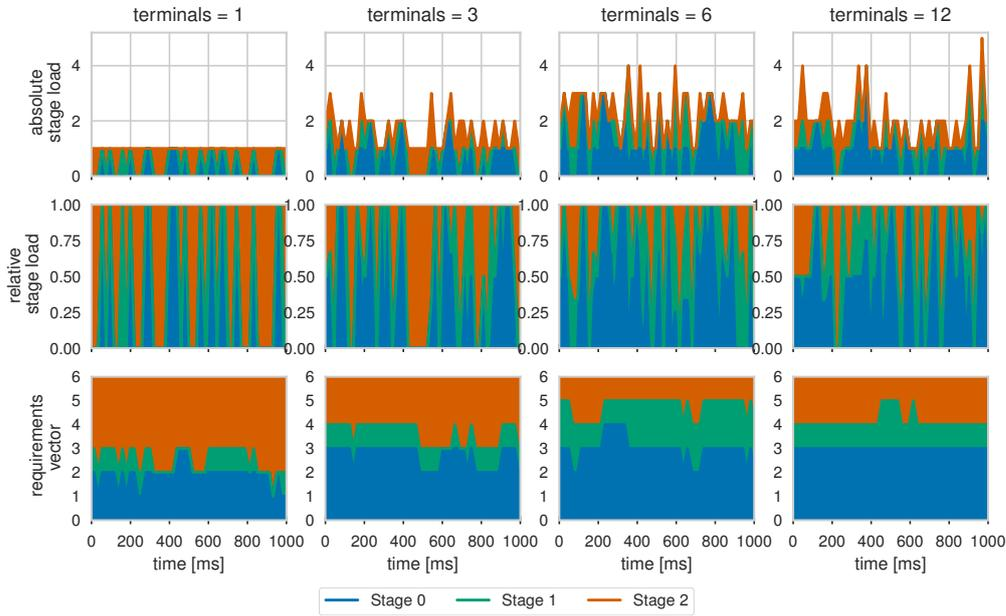
(a) Stage load and resulting requirements vector over time. The exponentially-decaying average filter smoothens the very spiky stage load profile.
