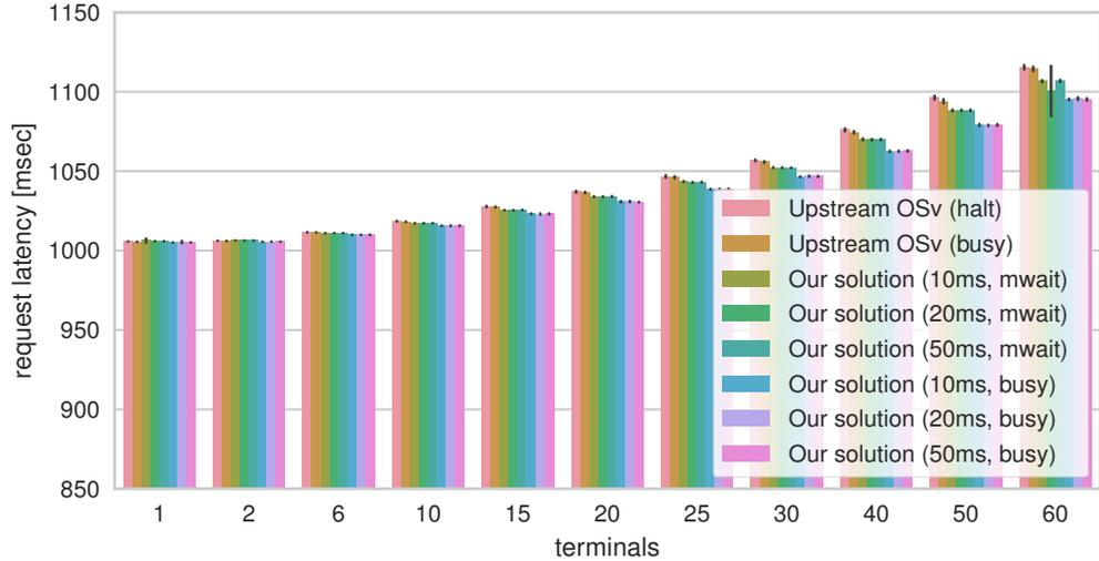
(b) TPC-C request latency. Our solution achieves up to 15ms lower request latency at 60 terminals. Note however that this is only 1.5% faster than upstream and that the y-axis in the diagram starts at 850msec.
