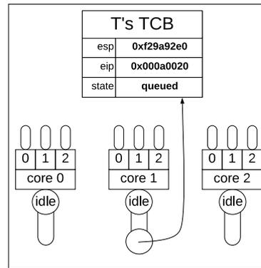
(d) The idle thread on core1 observes T in state stagemig\_sto and admits it to the ready queue.
