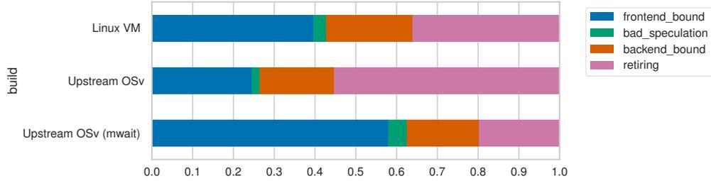
(a) Top-down analysis top-level breakdown. The true frontend-boundedness of MySQL on upstream OSv is only visible when removing spinning in the idle thread, which we did with the `mwait` configuration. The break-down corresponds to the observations made by Kanev et al. (Section 2.6).
