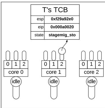
(c) T schedules out. The context switching routine sets its state to stagemig\_sto after T has stopped running on core2.
