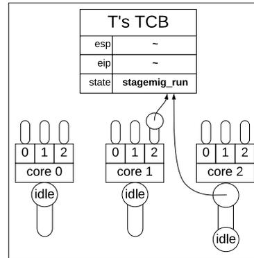
(b) T switches to stagemig\_run and puts a pointer to its TCB into the incoming migrations queue at core1. Core1's idle thread does not dequeue TCBs with state  $\neq$  stagemig\_sto.
