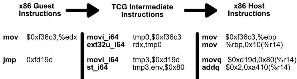
Figure 2.2: The guest's instructions are translated into the TCG's intermediate instruction format. From there on, they are further translated to the instruction set used by the host.
