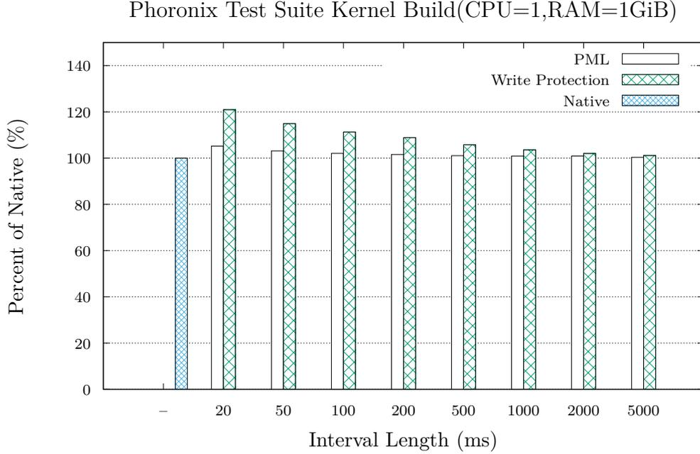
Figure 3.3: Comparison of time to completion of a Linux kernel build between PML and write protection. The horizontal axis denotes interval length between polling the dirty bitmap in milliseconds. The vertical axis denotes time to complete the benchmark, measured on the host, lower is better. The results show a similar progression to that of SPECjbb2005.
