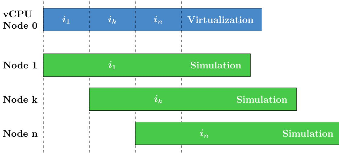
Figure 2.1: Acceleration of full system simulation via SimuBoost. The virtualization node runs the workload and creates checkpoints. Simulation nodes run simulations of intervals, with the respective checkpoint as starting state.
