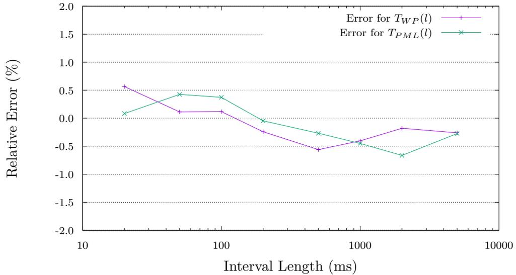
Figure 3.8: The relative errors of  $T_{WP}$  and  $T_{PML}$  to the measured values. Both are accurate to 1%.
