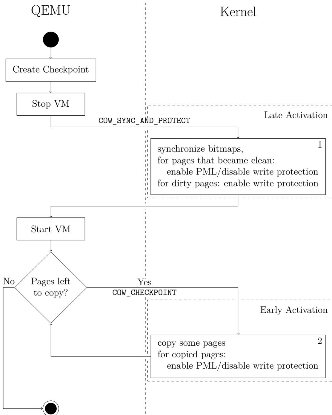
Figure 4.3: Overview of our modifications for PML activation. Late activations only requires changes to [\[1\]](#); early activation changes to [\[2\]](#).
