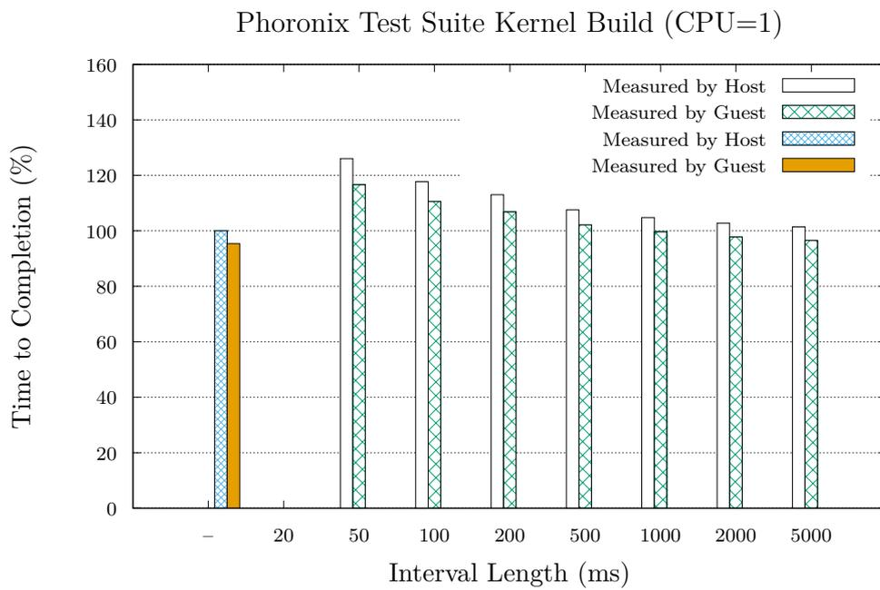
Figure 3.11: Time to complete a kernel build while performing checkpointing using write protection as dirty logging mechanism. Values are given in percent of native, measured by host, lower is better. Because of limited hardware, accurate measurements for an interval length of 20ms could not be obtained, as a result the value has been omitted
