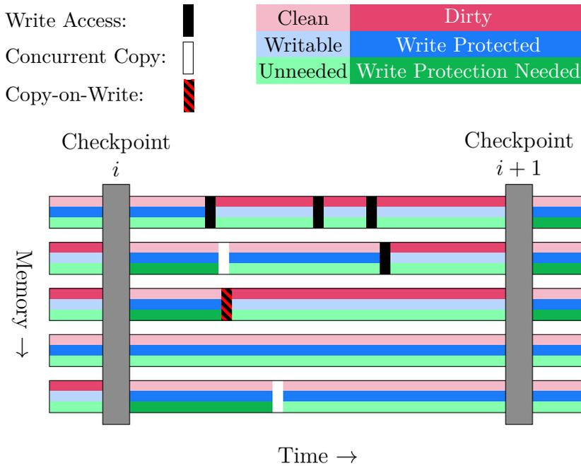
Figure 3.9: Overview of incremental COW checkpointing using write protection for dirty tracking. Write protection is enabled whenever a page is clear.
