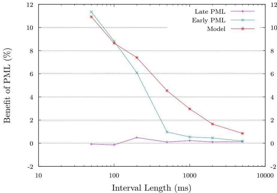
Figure 5.2: The benefit of late and early PML over write protection, as well as the predicted gain. Early activation achieves an improvement, the benefit of late PML is neglectable. The model severely overestimates the benefit for intervals  $\geq 500$ s.
