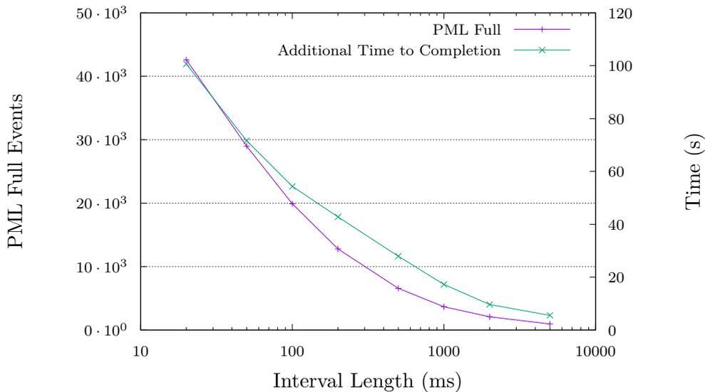
Figure 3.7: Comparison of PML full events introduced by dirty logging via PML compared to the additional time to complete a kernel build. The number of PML full events is given by the left y-axis, the time to completion on the right. Values given are for one CPU. Overall, the curves are similar but not as close as in the same consideration for write protection.
