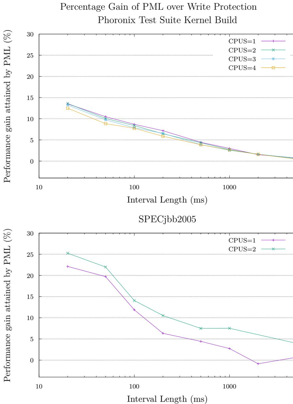
Figure 3.4: Overview of the performance increase created by PML. The horizontal axis denotes interval length on a logarithmic scale, the vertical axis denotes gain of PML over write protection in percent, higher is better. For interval lengths  $\geq 100$ ms, the increase varies between 14% and -1%. At an interval length of 2s and 1, CPU PML causes a decrease in performance, for reasons unknown.
