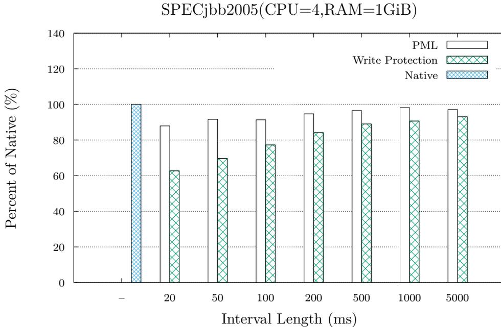
Figure 3.2: Comparison of performance in SPECjbb2005 running with four cores between no dirty logging and dirty logging with PML or write protection. The horizontal axis denotes interval length between polling the dirty bitmap in milliseconds. The vertical axis denotes score in SPECjbb2005, compared to native, higher is better. The results are very similar regardless of the number of CPUs.
