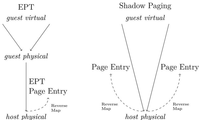
Figure 4.2: Comparison between two level paging (EPT) and shadow paging, when changing write protection. In the case of EPT, the page entry in the *guest physical*  $\rightarrow$  *host physical* table must be modified. In the case of shadow paging, all entries in *guest virtual*  $\rightarrow$  *host physical* tables must be modified. Going backward via the reverse map automatically performs the right action.
