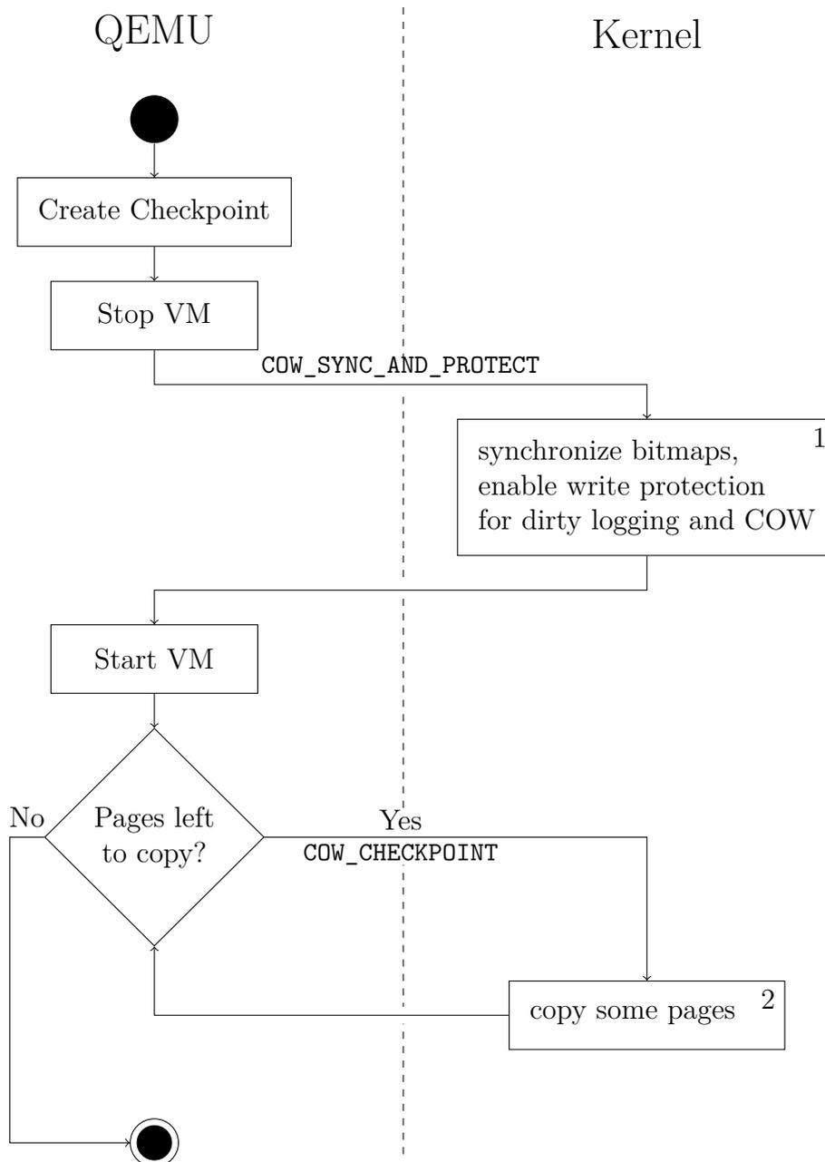
Figure 4.1: Overview of SimuBoosts checkpointing implementation. Elements on the left execute in user space, elements on the right in kernel space. **1** constitutes the work performed during the downtime. **2** is the majority of work, performed asynchronously to workload execution.
