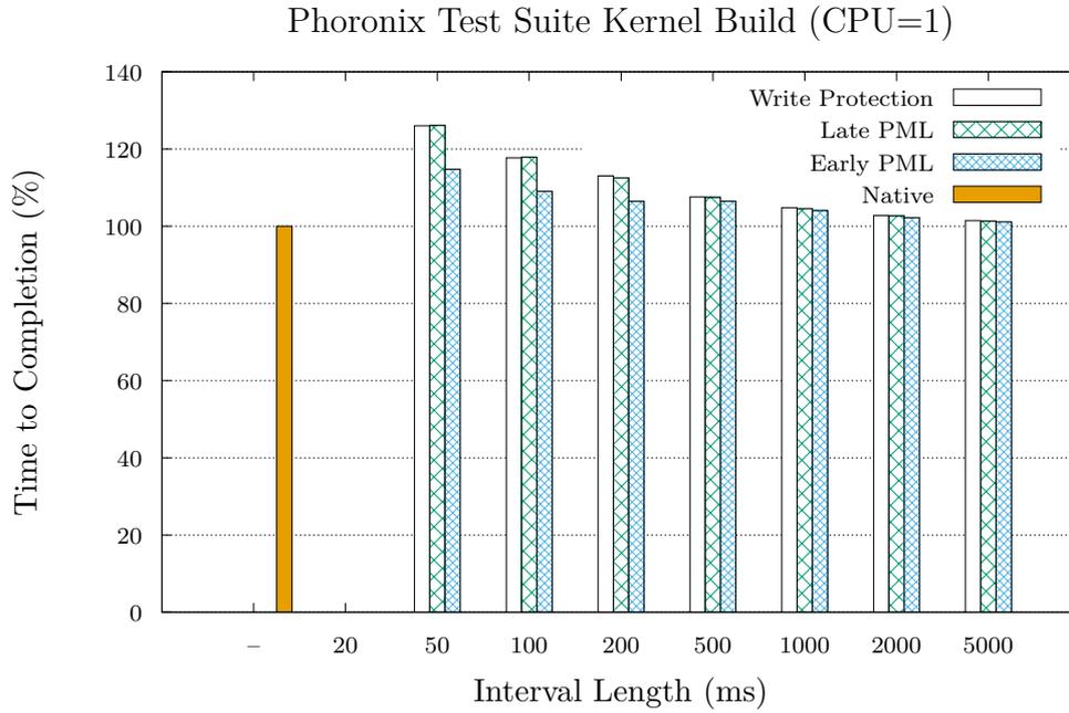
Figure 5.1: The measured time to complete a kernel build for all implementations. Values are in percent of native, lower is better. Write protection and late PML activation are very similar, early activation is able to decrease the run time.
