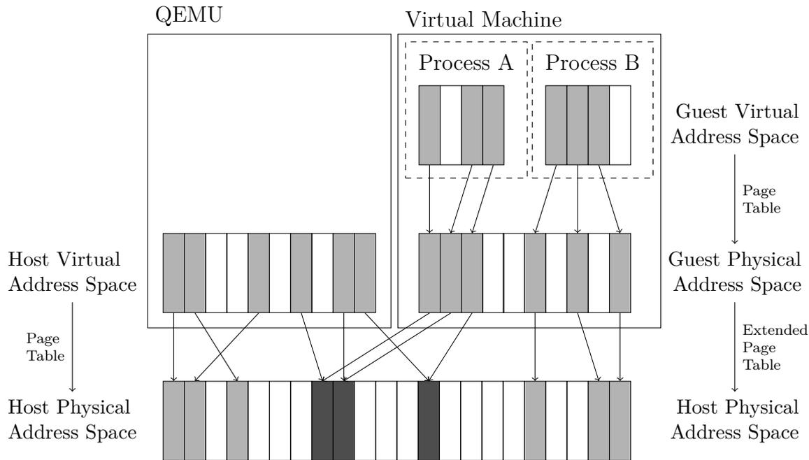
Figure 2.2: The KVM memory setup [20]. Guest virtual addresses are translated to host physical addresses. These translations are managed by KVM using two-dimensional paging if available (as shown), shadow page tables otherwise. QEMU can control the memory of the virtual machine by directing KVM to map the physical memory backing some region of QEMU’s virtual address space into the physical address space of the guest (■).
