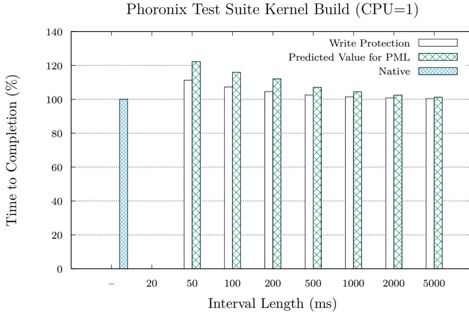
Figure 3.12: The time to complete a kernel build, while checkpointing, measured inside the VM, compared to the predicted time for PML. Values are in percent of native, lower is better. The value for 20ms has been omitted, because accurate measurements were not possible.
