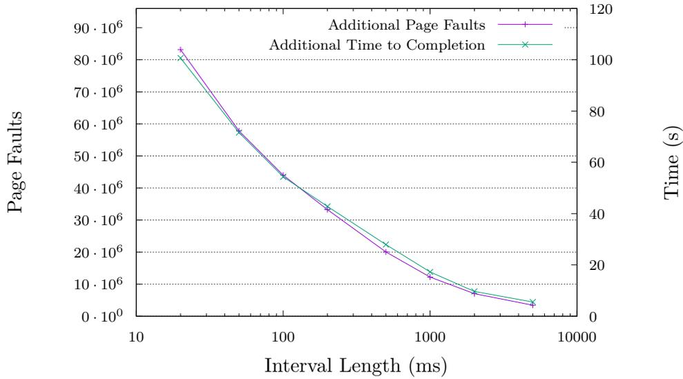
Figure 3.6: Comparison of page faults caused by dirty logging via write protection to the increase in time to complete a kernel build. The number of page faults is given by the left y-axis, the time to completion on the right. Values given are for one CPU. The curves show a similar progression, indicating that one can be predicted from the other.
