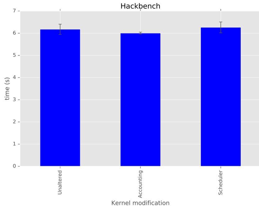
Figure 6.3: Hackbench results. Stresses the scheduler. Compares an unaltered kernel, one with the additional per process IO accounting, and one with the scheduler changes.
