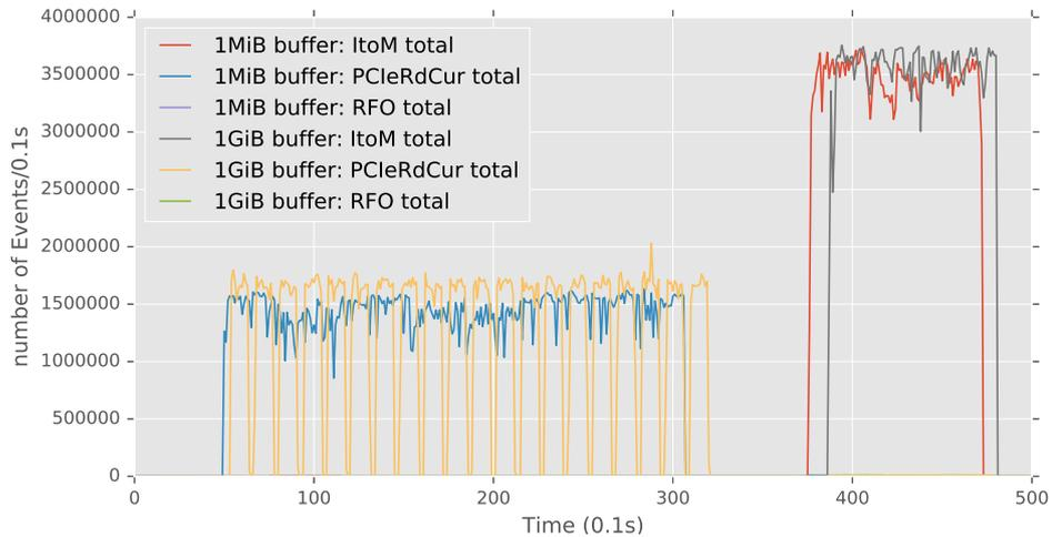
(a) Storage device benchmark. The benchmarks are run with different buffer sizes. With 1GiB buffers, the write benchmark has a pattern that follows the time a buffer is sent to the OS.
