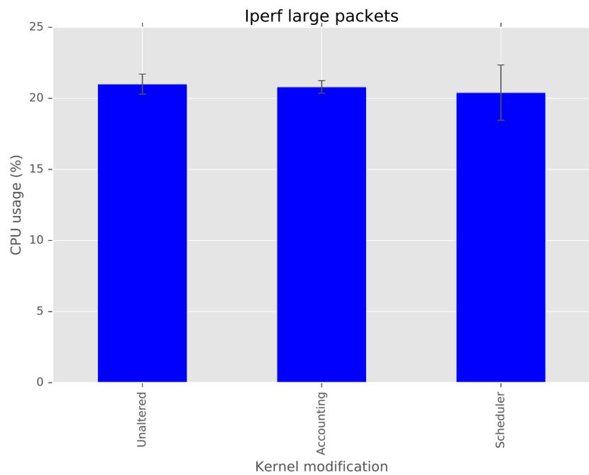
Figure 6.4: Iperf, with large packets. As the benchmark saturates the network this reports the CPU usage on an unaltered kernel, one with additional per process accounting, and one with the accounting and scheduler modifications.
