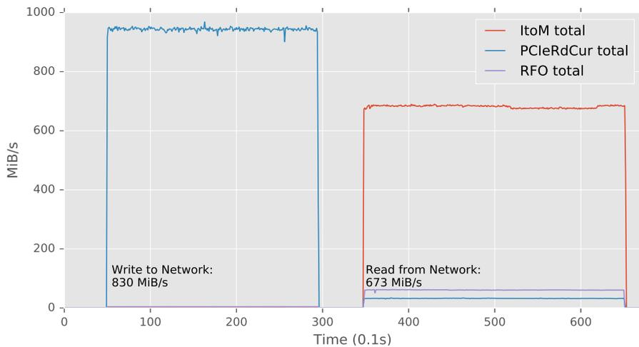
(b) Network benchmark. From 5s to 30s the benchmark writes to the network, from 35s to 65s the benchmark reads from the network.
