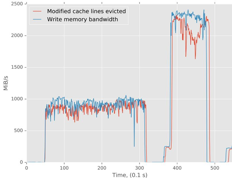
Figure 3.4: Comparison of the number of evicted modified cache lines with the write memory bandwidth reported by the memory controller. The bandwidth reported by the cache controller follows the bandwidth reported by the memory controller. The drift in the data is due to how the data was collected.
