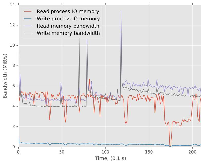
Figure 6.1: Total memory bandwidth compared to process IO memory bandwidth. The reported IO memory bandwidth is close to the total memory bandwidth. There is a slight difference in the data as it had to be gathered in separate runs. This demonstrates that the system provides plausible data.
