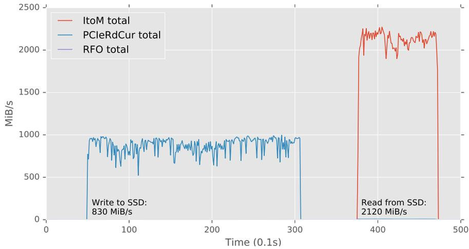
(a) Storage benchmark. From 5s to 32s the benchmark writes to disk, from 37s to 47s the benchmark reads from disk. RFO is too small to show on the scale
