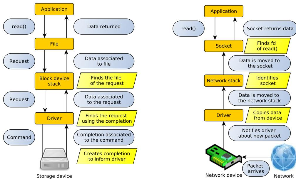
(a) Reads on storage devices cause the device to write data to memory
