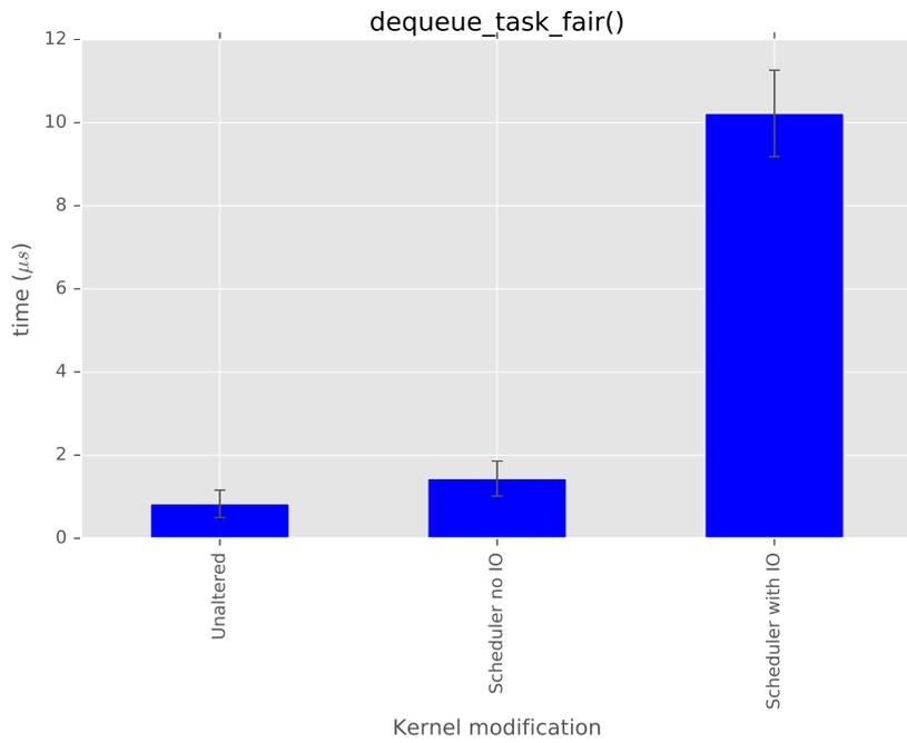
(a) Scheduler. Compares the latency of the same function to dequeue a process. Once on an unaltered kernel and twice on a kernel that implements updating process's IO memory bandwidth. In one case the process produces no IO and in the other it does.
