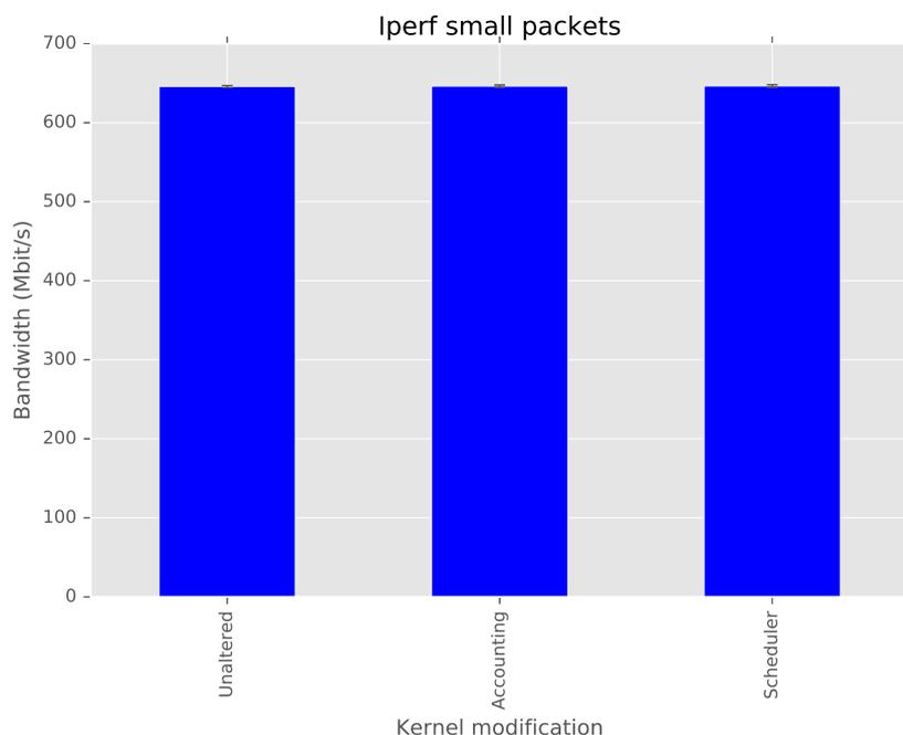
Figure 6.5: Iperf, with small packets. As the CPU is constantly at 100% utilization, this reports the Mbit/s bandwidth the benchmark achieves. The results are reported for a kernel without modifications, with only the accounting in the driver, and with the changes to the scheduler and accounting.
