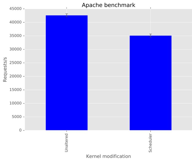
Figure 6.6: Apache benchmark. Reports the requests per second to a Apache 2.4 server on the test system. The server is run on a system with an unaltered kernel and on a system with the kernel implementing the scheduler and accounting modifications.
