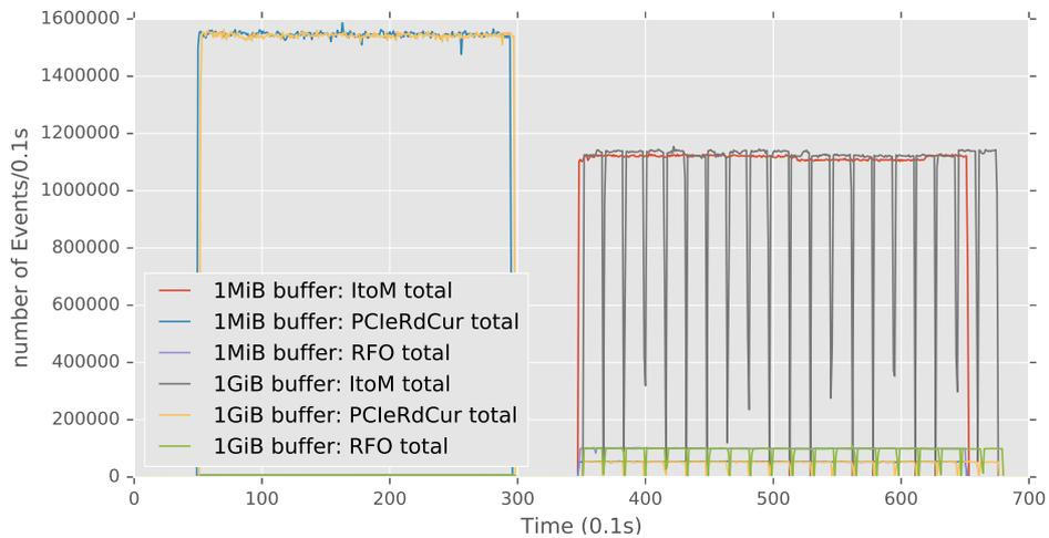
(b) Network device benchmark. The benchmarks use different buffer sizes. With 1GiB buffers, read benchmark has a pattern that follows the time when the buffer is sent to the OS on the sending machine.
