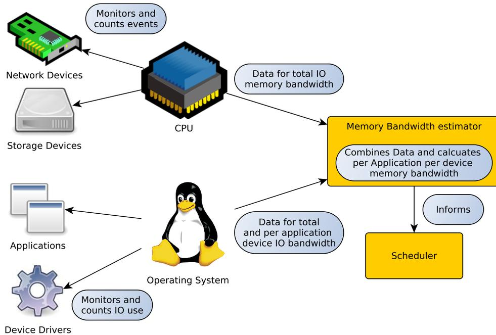
Figure 4.1: Overview of the IO memory bandwidth estimation system's design
