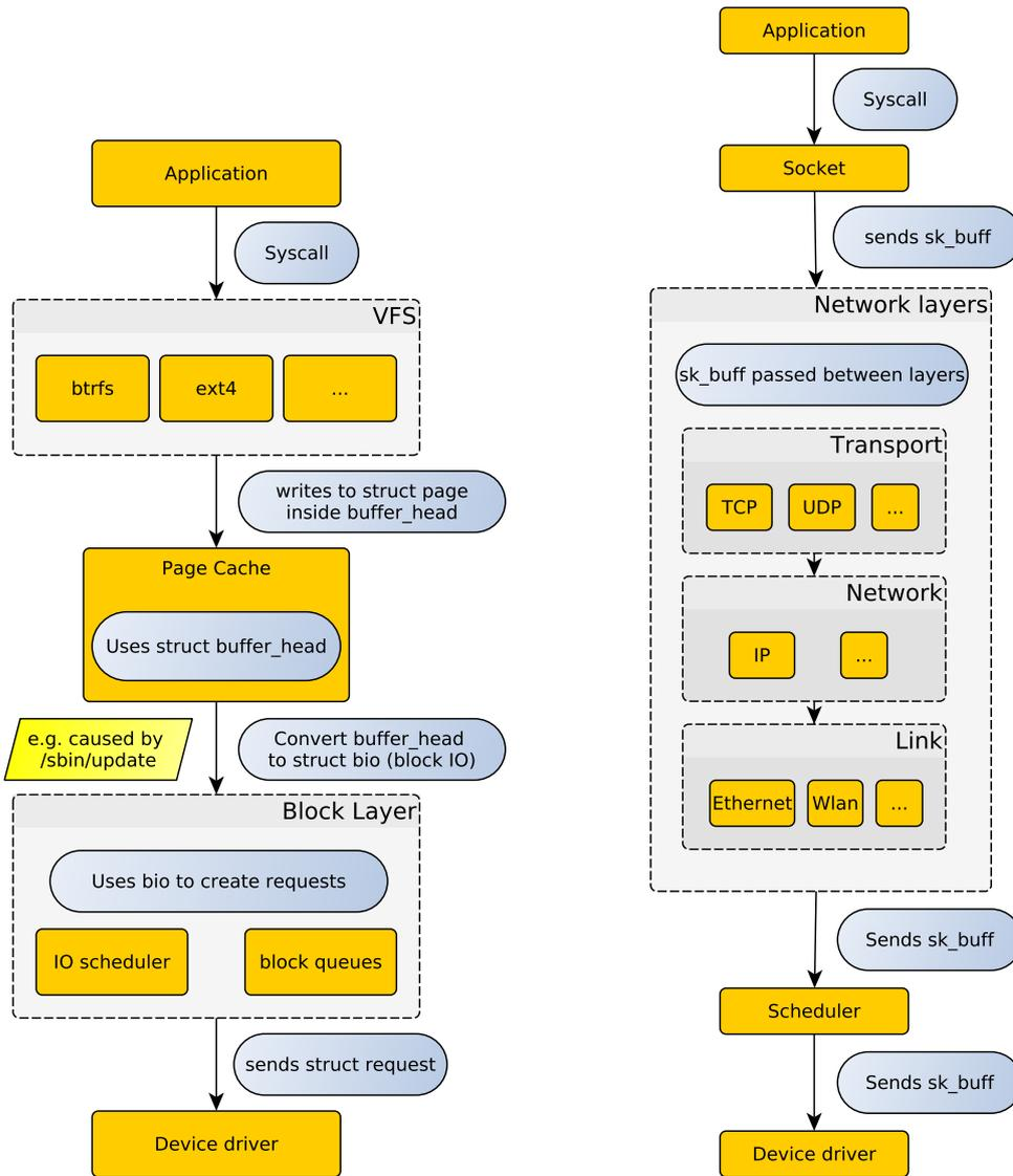
(a) Simplified part of the storage device stack in Linux. Different data structures are used in each step. Different programs can cause data from the page cache to be written to disk
