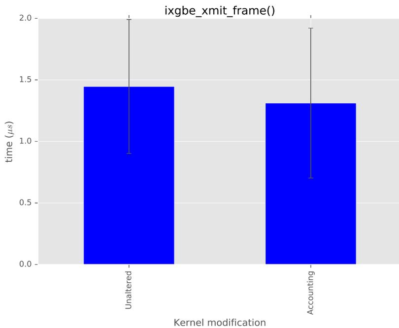
(b) 10Gbit Ethernet driver. Compares the latency of the Ethernet driver's transmit function in an unaltered kernel and in a kernel with additional accounting in the transmit function.
