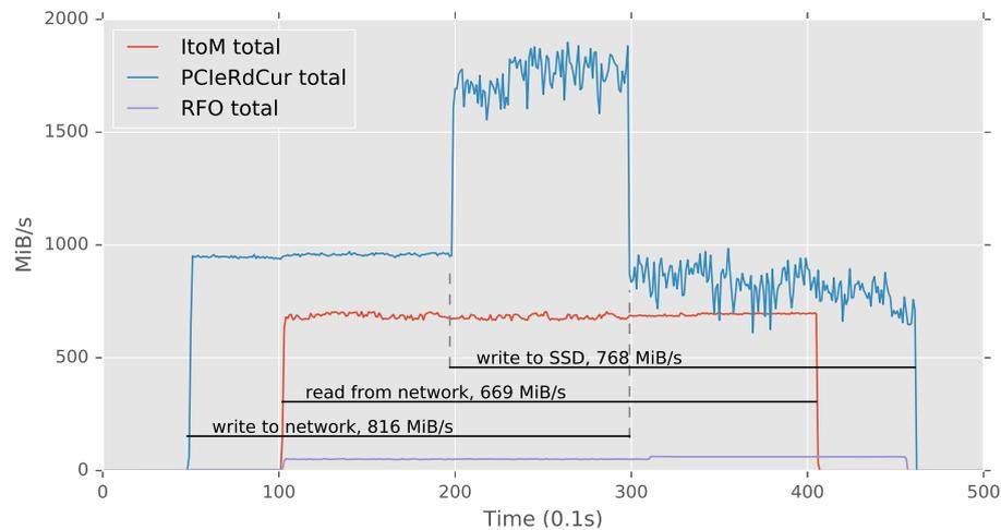
Figure 3.3: Events counted for TOR\_INSERTS filters. ItoM tracks writes, PCIeRdCur tracks reads from memory. RFO tracks partial writes. Network and storage benchmarks run simultaneously. The bandwidth reported by the counters follows the total bandwidth.
