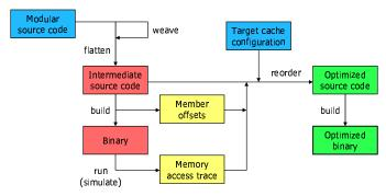
Fig. 2. The optimization embedded into the kernel build process. A kernel with flattened classes is built and profiled to collect access patterns on the critical path. In a second step, members in the flattened classes are reordered for optimal cache usage.
