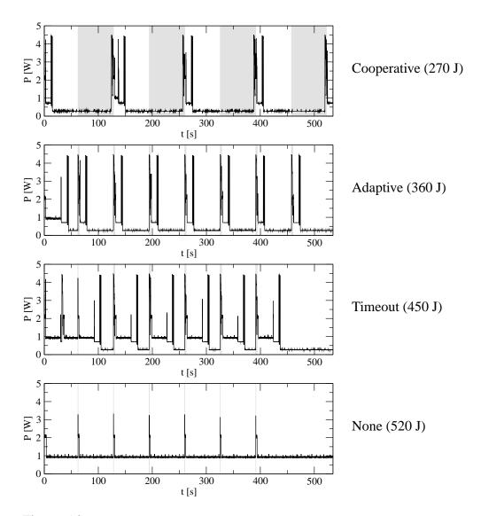
Figure 5.2: The hard disk's power inputs when playing "Toccata" using the four energy saving strategies. In the shaded regions, the program has called *read()* or *read\_coop()* and waits for its completion.
