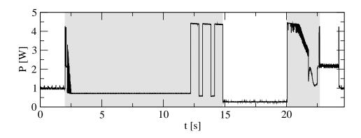
Figure 2.1: Power consumption of the IBM DCRA-22160 during an idle-standby-idle turnaround.
