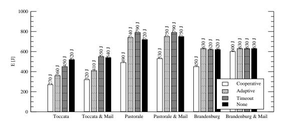
Figure 5.1: Energy consumption for three sound files played with four different policies.
