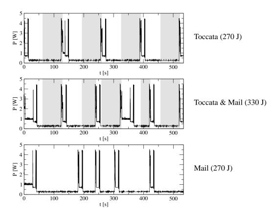
Figure 5.3: The hard disk's power inputs when playing "Toccata", receiving Mail or doing both using Coop-I/O. In the shaded regions, the MP3 player has called *read\_coop()* and waits for its completion.
