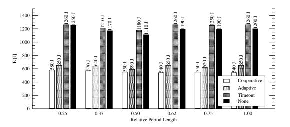
Figure 5.6: Energy consumption for five write processes, varying the period length.
