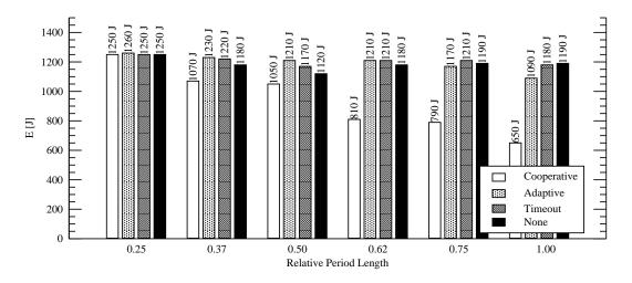
Figure 5.5: Energy consumption for five read processes, varying the period length.
