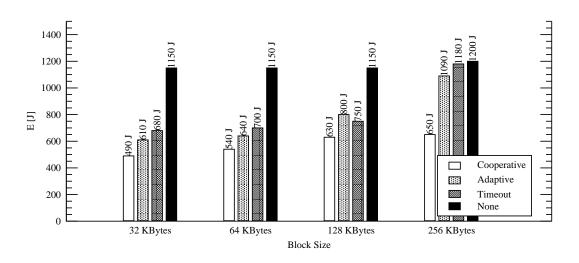
Figure 5.8: Energy consumption for five read processes, varying the block size.
