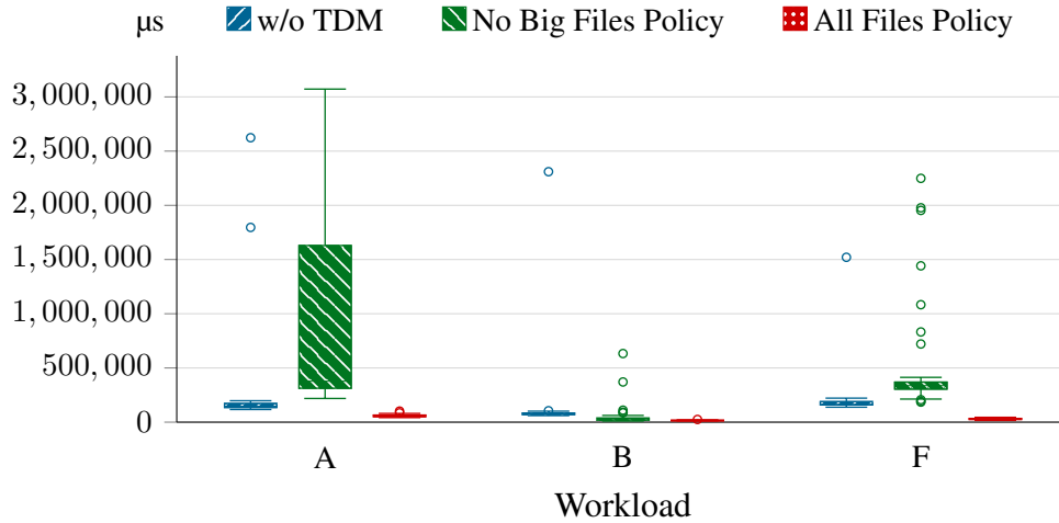
Figure 5.5: Box plot over the maximum update latencies of all 50 runs. Each box spans the interquartile range (IQR). Whiskers reach the furthest sample within 1.5 times the IQR and circles mark outliers beyond it. No Big Files Policy causes higher latencies and more outliers in most of the workloads. With workload A, the high latencies under the No Big Files Policy are so frequent that all samples lie within 1.5 times the IQR.
