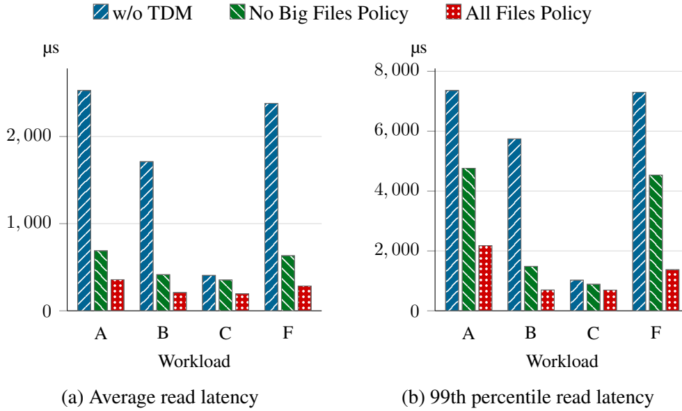
Figure 5.2: Read latency reported by YCSB across the evaluated workloads and policies. Lower is better. The All Files Policy (4.1.1) has the lowest average and 99th percentile read latencies.
