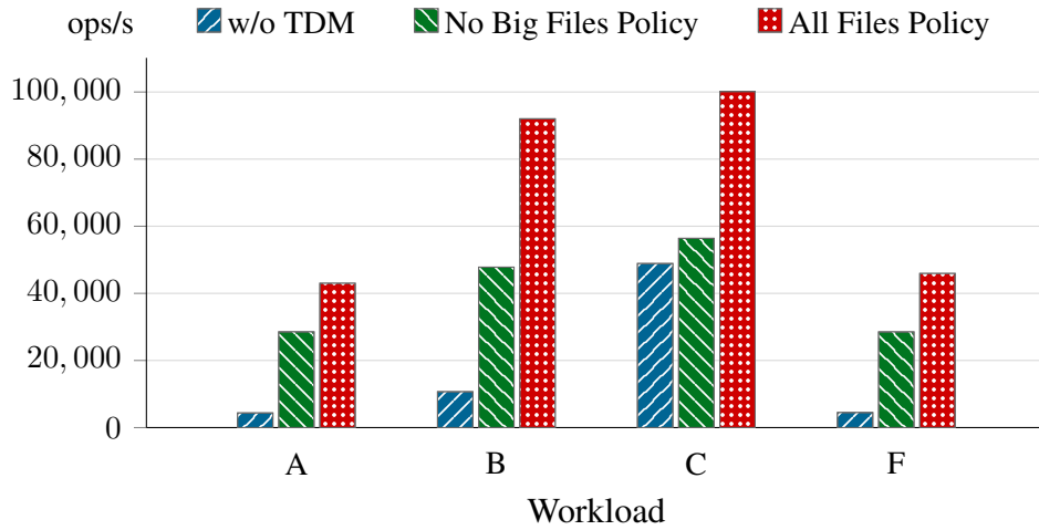
Figure 5.1: Throughput reported by YCSB across the evaluated workloads and policies. Higher is better. The All Files Policy (4.1.1) achieves a speedup of up to 10 times with workloads A and F. The No Big Files Policy (4.1.2) achieves a speedup of up to 6.5 times with these workloads.
