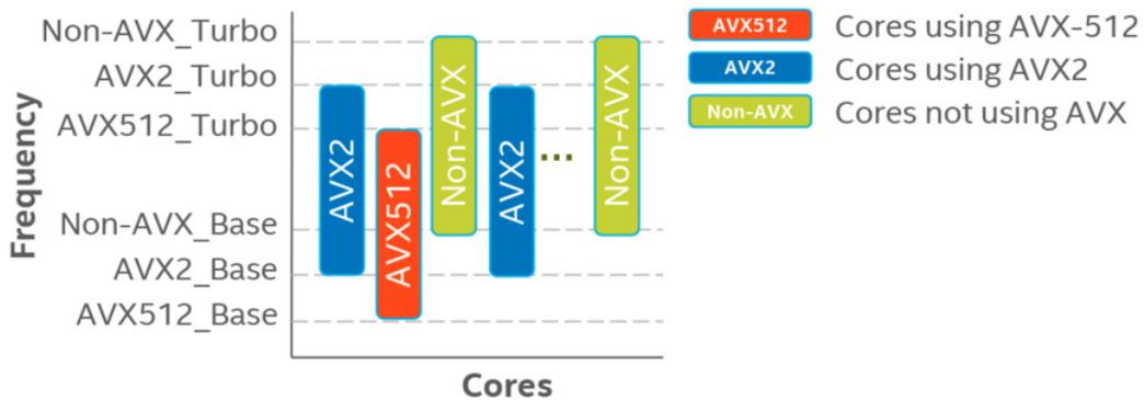
Figure 2.3: Intel Skylake-SP processors have different (lower) frequency ranges for the vector instruction set extensions AVX2 and AVX-512 [wika].
