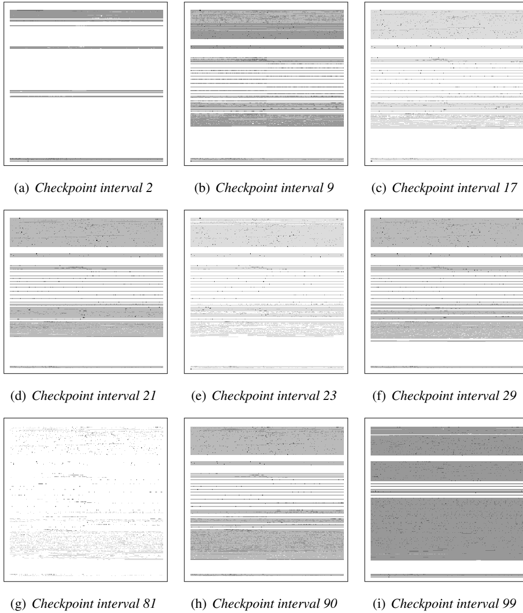
Figure B.4: Access patterns of a Linux kernel build with a checkpoint interval length of 8000 ms.
