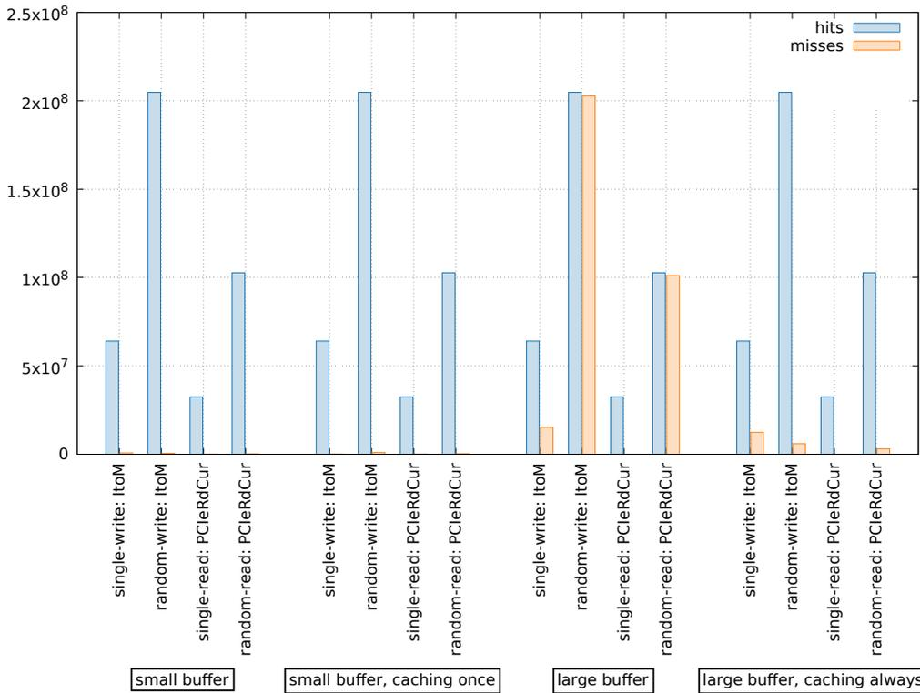
Figure 5.7: Comparison of PCM event counts with different buffer sizes and caching modes in `nvme-memload`. Only events including transferred data blocks are shown.
