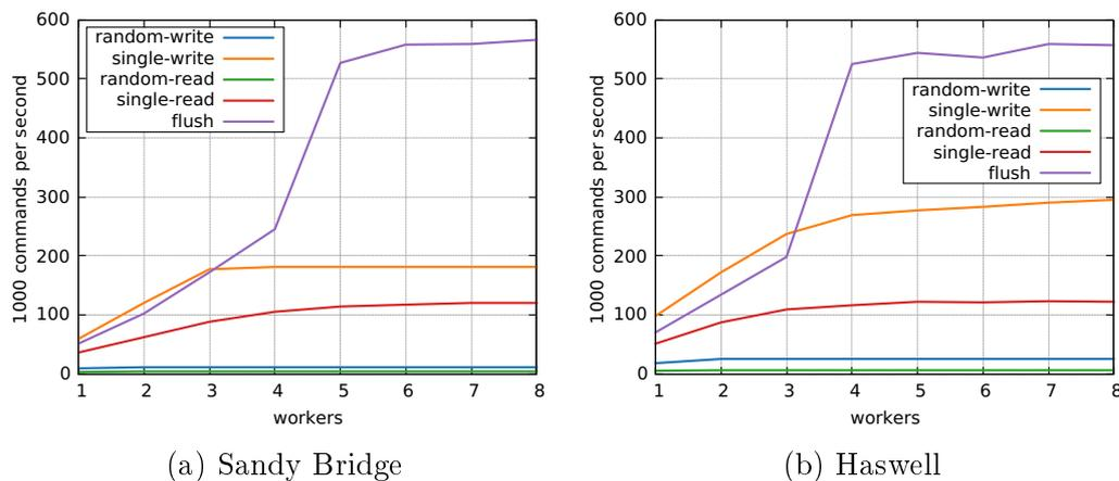
Figure 5.2: NVMe command rate of `nvme-memload` with different amounts of worker threads.
