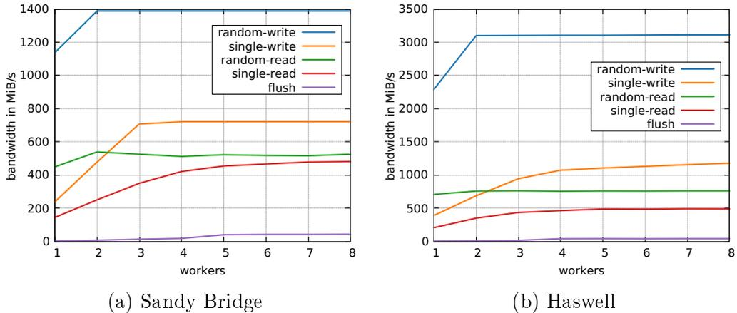
Figure 5.1: DMA bandwidth used by `nvme-memload` with different amounts of worker threads sending NVMe commands.
