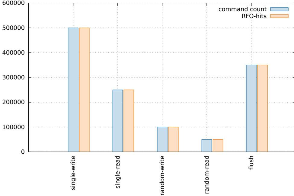
Figure 5.5: Comparison of the command count and RFO-hits events for each pattern.
