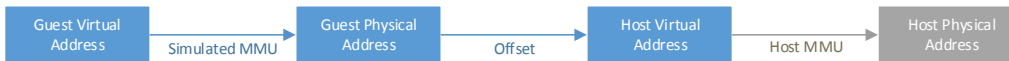
Figure 2.2: The simulator translates guest virtual to guest physical addresses by simulating a MMU in software. The subsequent translation (e.g., adding an offset) redirects the access to a guest physical address to an address within an area of the simulator's virtual address space which contains the guest's physical RAM content. The host's MMU can translate the resulting host virtual addresses to host physical ones, just like it does it for every other virtual address the simulator's code accesses.
