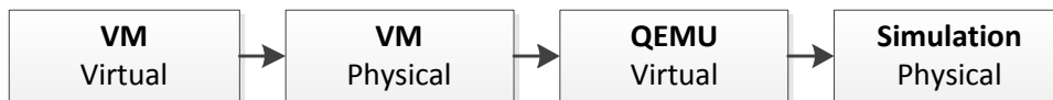
Figure 4.7: Three-Stage Address Translation. To access the payload buffer in a virtual machine, the tracer has to perform multi-level address translation.
