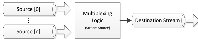
Figure 4.13: Stream Multiplexing. Multiple source streams are combined into a single output stream.
