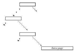
Virtual addresses are transformed step by step into real addresses by means of a page table tree. Let us consider an individual transformation step of a virtual (binary) address v for an action x by means of a page table with the address p. For this purpose, v is split into a high part u (consisting of a specific number of high bits) and a low value part v' (consisting of low bits). Using u, we select an entry of the page table including an access attribute u and a new address u.
