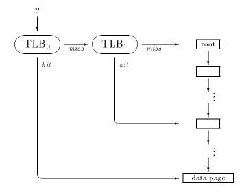
$TLB_0$  is a more or less conventional TLB on page basis or a virtual-addressable cache; a hit delivers the corresponding real address directly.  $TLB_1$  operates on larger regions (e.g. 16 MB) so that entering into the page table tree transversally is possible upon a near miss ( $TLB_0$  miss and  $TLB_1$  hit), and only a small part of the tree has to be parsed.
