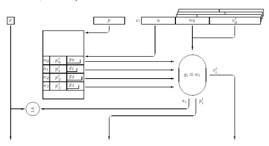
Here, the 4 selected entries are read in parallel and analyzed (in parallel). It is to be noted that the guards  $g_i$  usually differ with regard to their lengths, i.e. for the various comparisons, the bit string reduced by u is divided into different pairs  $w_i, v'_i$ .
