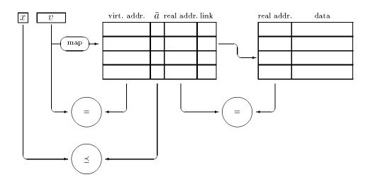
Here, field  $\bar{a}$  contains the resulting access attribute which is obtained from the combination of the access attributes of the individual levels during address transformation.
