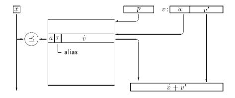
Address transformation is restarted with the resulting  $\dot{v} + v'$  which is a virtual address of full length. Consequently, the entire virtual region covered by the alias entry is mapped *virtually* to another virtual region:
