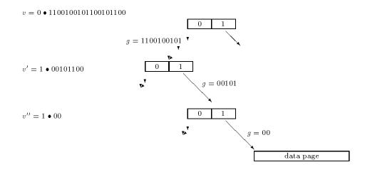
Each page table entry contains not only the pointer to the next level table (in the part denoted by p), but in addition a size specification s for this object. In the case of page tables, s refers to the number of entries; all powers of 2, i.e.  $1,2,4,8,\ldots$ , are admissible. The length of u is obtained from the current page table size.
