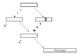
Unlike *real* aliasing, *virtual* aliasing is independent of real memory mapping. In this way, it enables modifications of mapping by means of user level software
