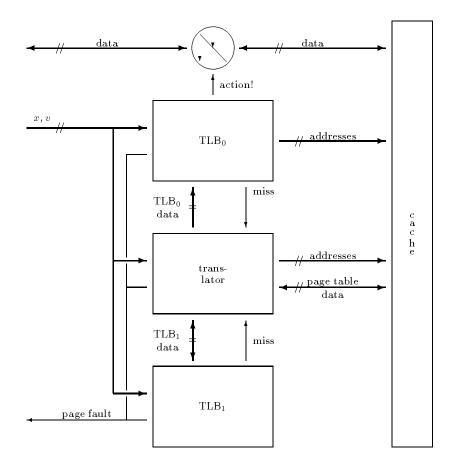
${\rm TLB_0}$  and  ${\rm TLB_1}$  are available here as independent hardware. Instead of the cache, a normal memory could of course be connected also directly.
