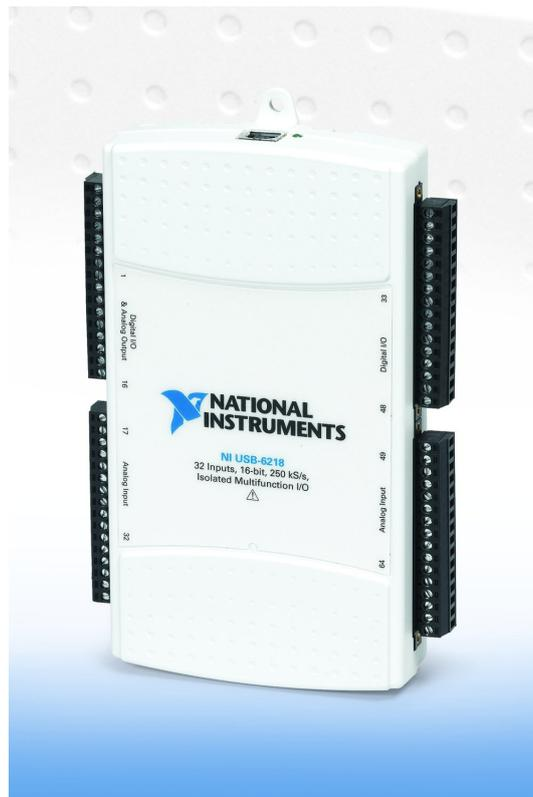
Figure 3.5: NI USB-6218 (picture from <http://www.pressebox.de/pressemeldungen/national-instruments-germany-gmbh/boxid/75241>)
