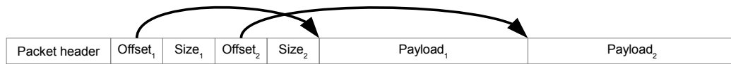
Figure 3.3: Layout of a short message packet. The header fields in front of the payload are fixed-size and can therefore be processed efficiently.
