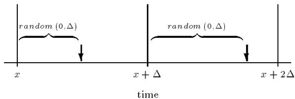
Scheduling remains the job of the periodic clock handler. Clock updates happen with the same frequency but are decoupled from the periodic interrupt. For implementation, we use two hardware timers, one periodic clock and a programmable timer:
