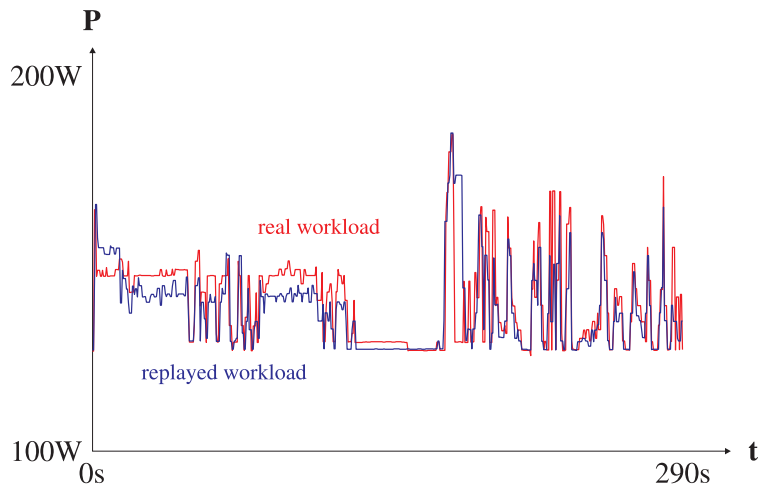
Figure 17: Power consumption of a file sync. Prediction error is 1.4 %. Hardware CPU: Intel Pentium D 3 Ghz, Memory: 2 GB, Network: Intel e100. Disk: Samsung HD080HJ Software rsync with compress option. Load Syncing and resyncing two linux kernel source trees and 4 big files.
