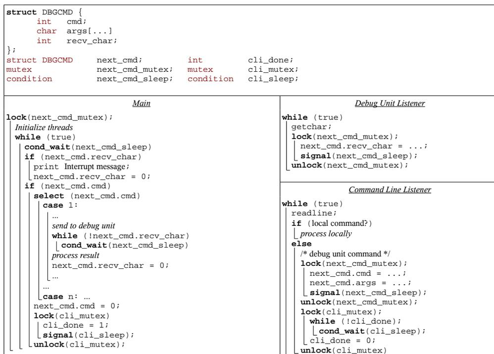
Figure 4.6: Pseudo code structure of the implemented debugging software
