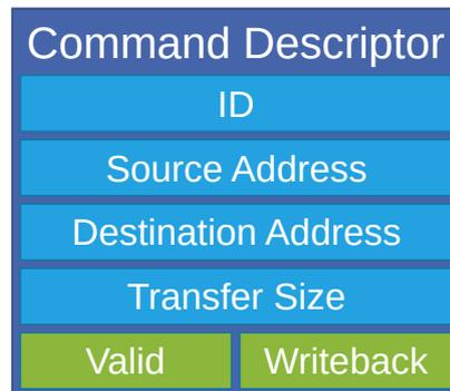
Figure 3.4: The contents of a command descriptor, as stored in the ring buffers that were previously configured via the QCSR. In the case of write (host-to-device) commands, *source address* references an address in the system memory, and *destination address* is handed to the FPGA-side user logic. The opposite is true for read (device-to-host) commands.
