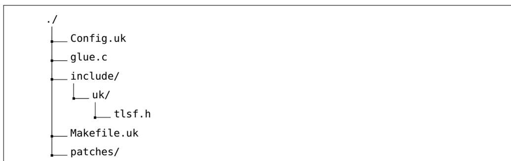
Figure 4.3: Unikraft library directory in the case of TLSF. The port skeleton comprises Unikraft build data, glue code, and patches for the allocator source.
