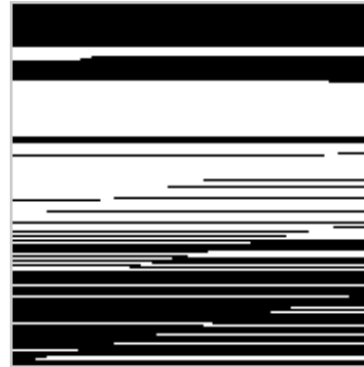
(d) Equivalent dirty memory if dirty logging had large page granularity. A coarser granularity leads to more dirty memory.
