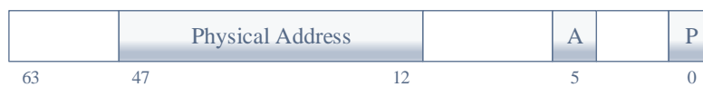
Figure 2.2: Scheme of the IA-32e architecture page table entry format for 4 KiB pages.
