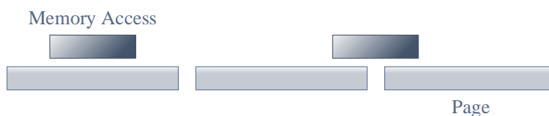
Figure 3.5: Two example memory accesses operating on three adjacent pages. The diagram depicts memory accesses as dark rectangles, pages as light rectangles. The width of the rectangles denotes the hypothetical size of both accesses and pages. The left memory access does not causes only a single page references as all data is located on a single page. The second memory access causes references to two adjacent pages since the data is spread on both pages.
