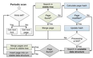
Figure 4: The high-level workflow of our new hint processing loop. When all hints have been processed before the scan rate is exceeded, XLH continues with the linear KSM scan to keep the rate constant.
