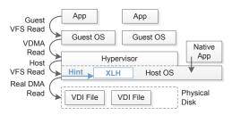
Figure 2: Host-VFS read and write operations are used to trigger hints for the main memory scanner.
