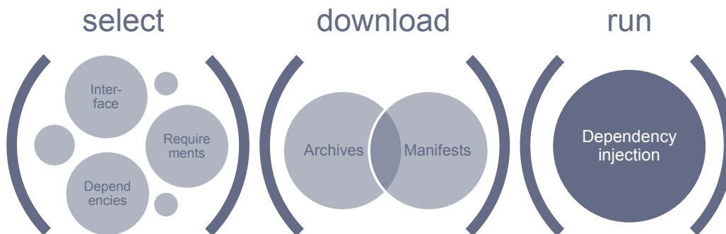
Figure 2.2: The Zero Install launch process is split into the phases select , download and run . Each phase depends on the results of the previous one.
