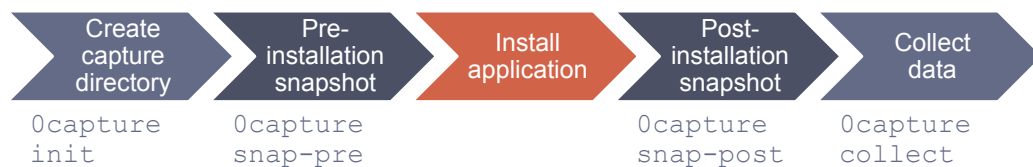
Figure 5.1: The 0capture command provides a set of sub-commands that are called in a specific sequence to capture the installation of an application.
