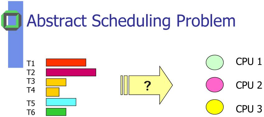
*How to assign these 6 threads to 3 CPUs? Is there an optimal schedule?*
