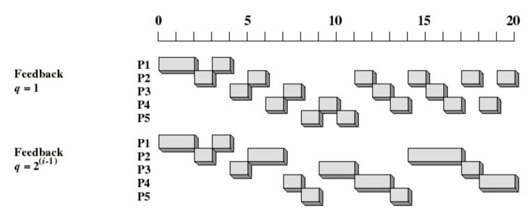
With fixed time quanta turnaround times of long threads can stretch out alarmingly, i.e. average turnaround time of long runners increase  $\Rightarrow$
