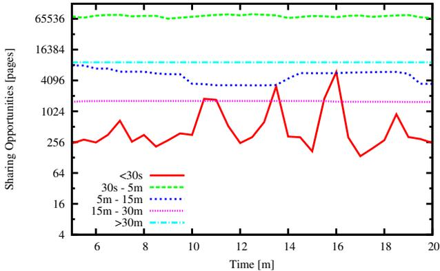
**Figure 1.** The longevity of sharing opportunities between two VMs that are compiling Linux v3.0. Notice the logarithmic scale. Sharing opportunities that last between 30 sec and 5 min are by far the most common.
