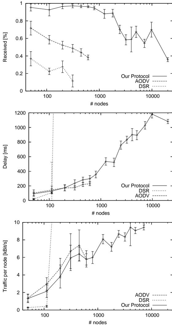
Figure 5: Hybrid MANETs with 1% fixed-wired nodes
