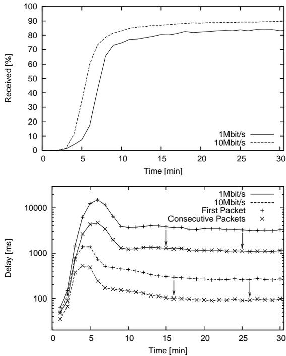
Figure 14: Variation of line speed for fixed-wired links
