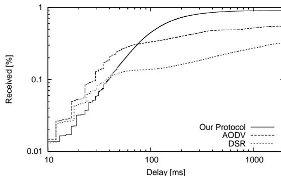
Figure 7: CDF of the end-to-end delays
