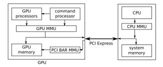
Figure 1. Memory access paths in a system consisting of a CPU and a GPU
