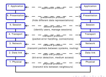
A Brief Introduction to Networks The Network Layer (3) The Transport Layer (4) Introduction Layered Communication Layers in the ISO/OSI Model
