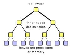
• Upper levels with higher bandwidths or multiple redundant links
