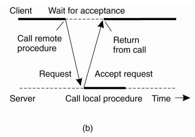
The interaction using asynchronous RPC
