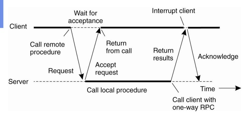
Client & server interacting with 2 asynchronous RPCs
