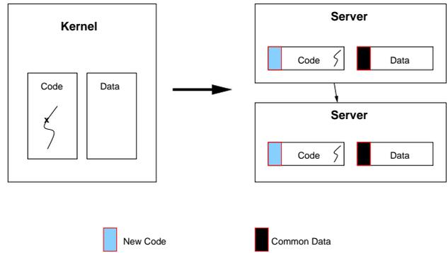
Figure 1: Decomposing a monolithic operating system into a multiserver operating system involves: (1) additional communication between servers; (2) buffer management for common data in multiple tasks; and (3) the addition of new code to compose a system from independent servers.
