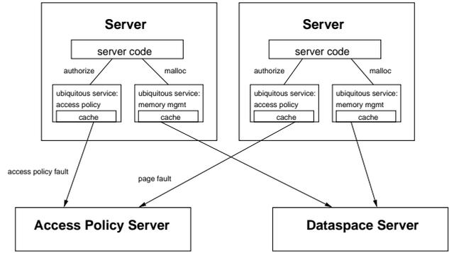
Figure 2: The SawMill approach enables the decomposition of monolithic operating systems into individual *system servers* where *ubiquitous services* manage server data obtained from *resource servers* locally.
