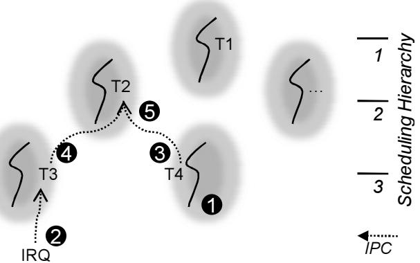
Figure 4: Recursive Preemption Message Chain. While executing (1), T4 is preempted by an interrupt delivered to T3 (2). It sends a preemption IPC to its scheduler T2 (3); since T2 is a scheduler of T3 as well, T3 also sends a preemption IPC to T2 (4), and T2 starts executing (5).
