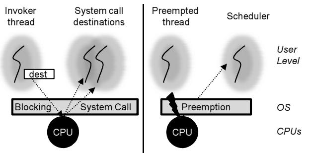
**Figure 1: User-Level Scheduling Design.** The kernel treats blocking system calls as implicit control transfers; the invoker resolves scheduling ambiguities by selecting the destination thread. Preemptions translate into notifications of a user level scheduler.
