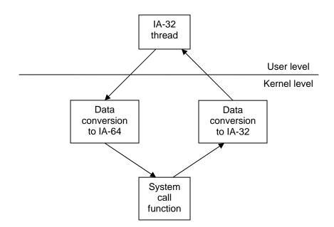
Figure 4.13: Communication between an IA-32 thread and the kernel
