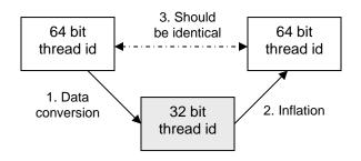
Figure 4.14: Thread id conversion test
