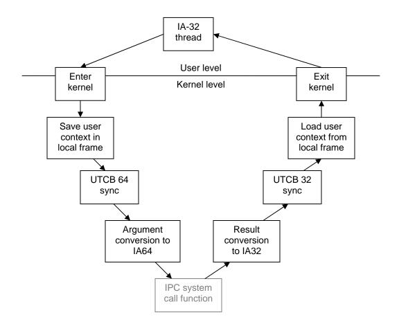
Figure 5.2: IPC system call stub for IA-32 emulation layer
