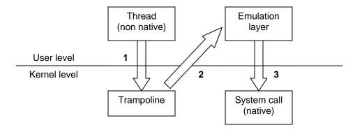
Figure 3.9: The trampoline mechanism
