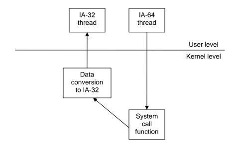
Figure 4.16: An IA-64 thread sending an IPC to an IA-32 thread
