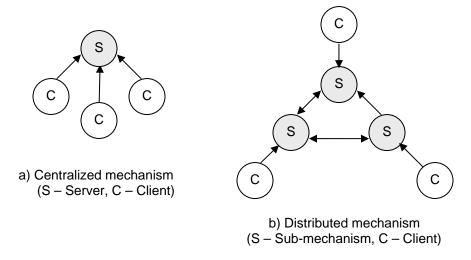
Figure 3.15: Architecture of coherency mechanisms
