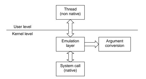
Figure 3.11: Emulation layer placed on top of the kernel
