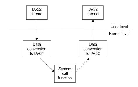
Figure 4.17: An IPC between two IA-32 threads
