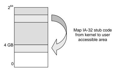
Figure 4.18: Mapping of IA-32 system call stubs
