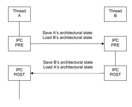
Figure 5.5: IPC operation between two IA-32 threads
