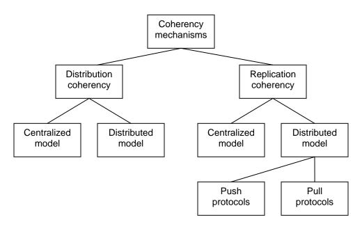
Figure 3.16: Classification of coherency mechanisms
