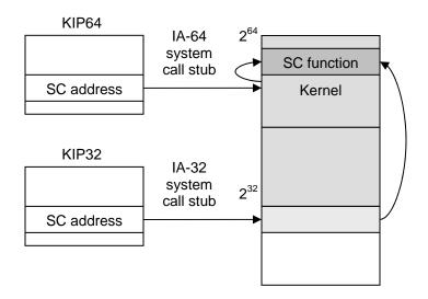
Figure 4.19: Coexistence of two KIPs
