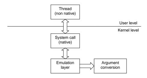
Figure 3.12: Emulation layer placed on bottom of the kernel
