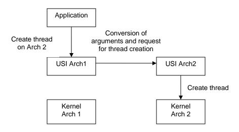
Figure 3.5: Creating a thread on a different architecture
