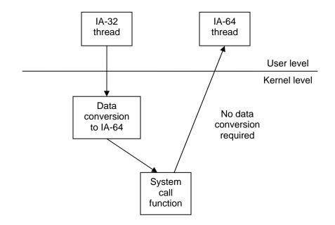
Figure 4.15: An IA-32 thread sending an IPC to an IA-64 thread
