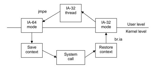
Figure 4.9: System call performed by an IA-32 thread
