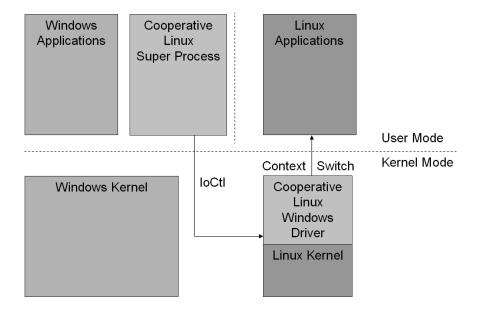
Figure 3.2: Cooperative Linux Design. The Super process frequently calls the Cooperative Linux driver via IoCtl. The driver then switches the complete context of the CPU to the virtualized Linux.
