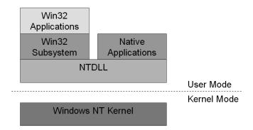
Figure 2.2: Native Applications. Native applications run directly on the NTDLL library. Win32 applications run on the Win32 API which in turn is a subsystem of the NTDLL library.
