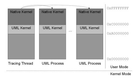
Figure 3.1: User-Mode Linux Design. The tracing thread is responsible for redirecting signals to UML processes and for tracing system calls from UML processes.
