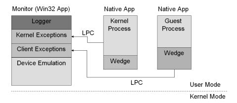
Figure 4.1: Windows NT Native VMM Design. The Monitor itself is a Win32 application, the guest OS kernel and processes run as native applications. They communicate with each other via named ports. The guest OS kernel and processes output to the logger using LPC. Exceptions and software-generated interrupts are sent via the exception port to the responsible exception handling thread by the underlying Windows NT system.
