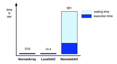
Figure 6.2: Measured execution time for accessing an array element 500 000 times
