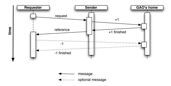
Figure 5.10: The implemented solution of exchanging references
