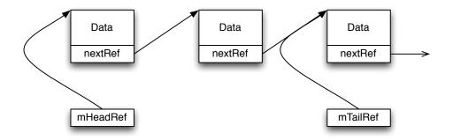
Figure 5.3: Link structure in a cQueue
