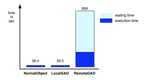
Figure 6.1: Measured execution time for accessing an object's field 1 000 000 times
