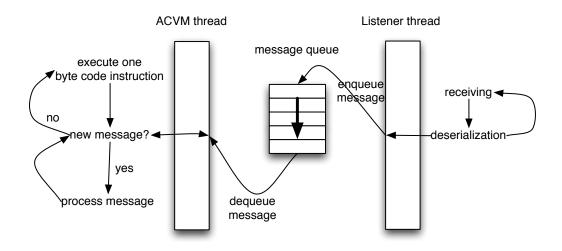
Figure 5.5: Both system threads and their processing loops
