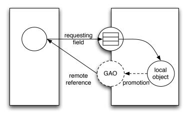
Figure 4.13: Accessing a local object through a reference from a GAO
