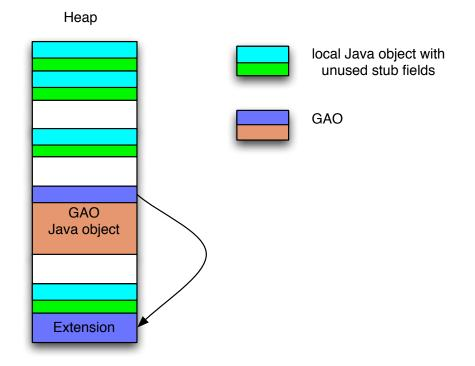
Figure 4.9: Heap structure with object extension enabled
