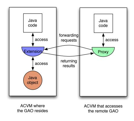
Figure 4.1: Components of a GAO
