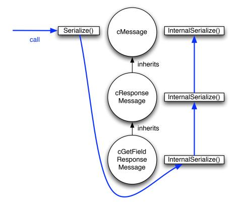
Figure 5.8: Message serialization structure
