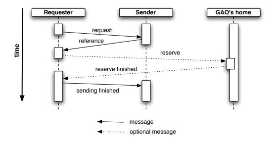
Figure 4.12: Safely transferring a reference to a GAO
