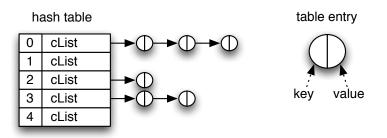
Figure 5.2: Link structure in a cHashtable
