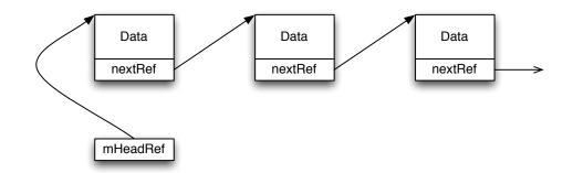
Figure 5.1: Link structure in a cList
