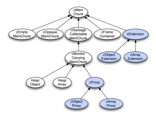
Figure 5.9: Inheritance hierarchy of MemChunks including extensions and proxies
