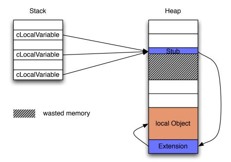
Figure 4.7: Object promotion by replacement with stub
