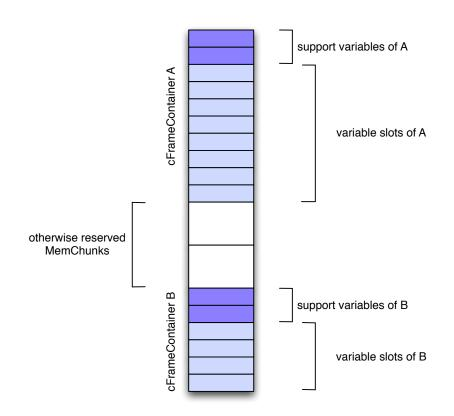
Figure 3.3: Two Java stacks allocated in memory
