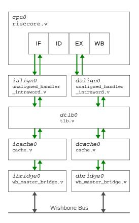
Figure 2.2: Standard memory access chain of the OpenProcessor
