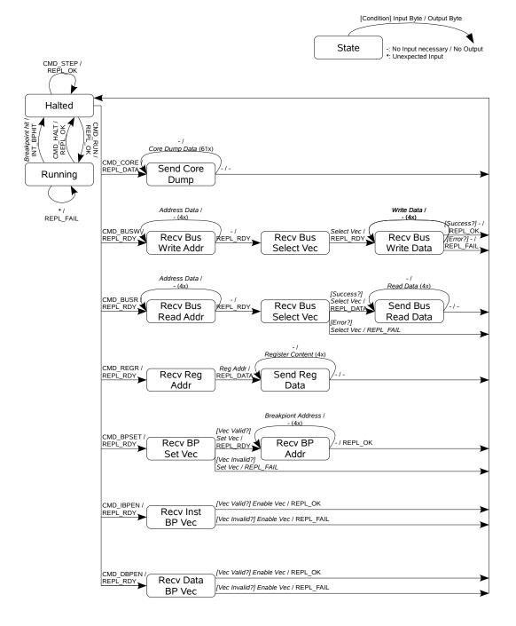
Figure 3.1: The debugging state machine and communications protocol, as seen by the user
