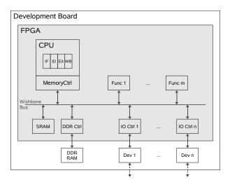
Figure 2.1: Logical view of the OpenProcessor Platform
