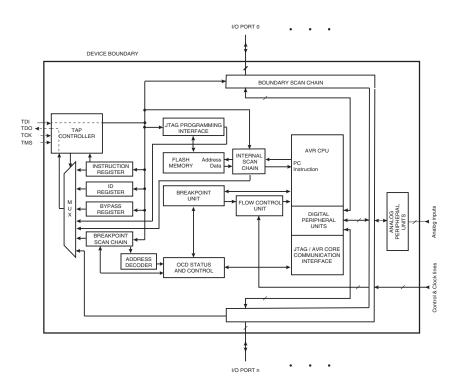
Figure 2.4: Block diagram of the JTAG test access port on the megaAVR [1]
