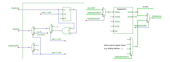
Figure 4.3: Stall logic for debugging
