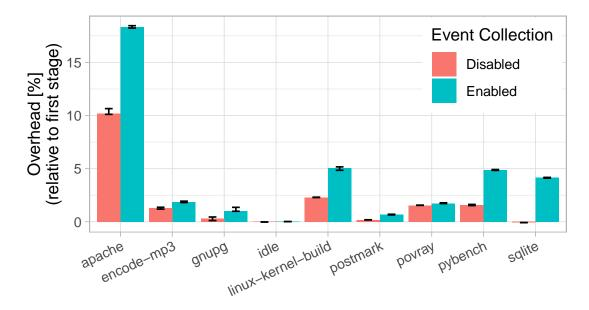
Figure 6.5: The event collection can impose a significant overhead on the replay. In some cases it more than halves.
