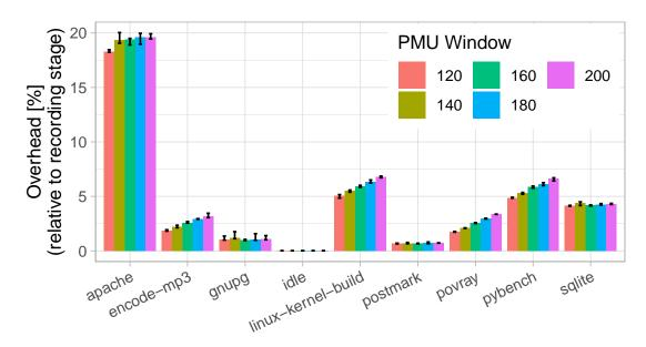
Figure 6.4: Our replay engine has an overhead of about 5% for most workloads compared to the recorded execution. Only Apache, which produces a large amount of events, incurs an overhead of 18%.
