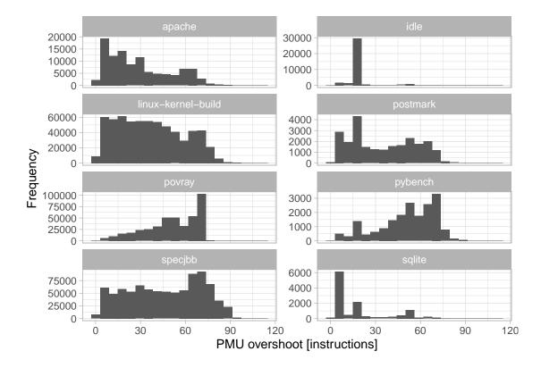
Figure 6.3: The histogram shows that the delay between performance counter overflow and interrupt arrival stays below 114 instructions.
