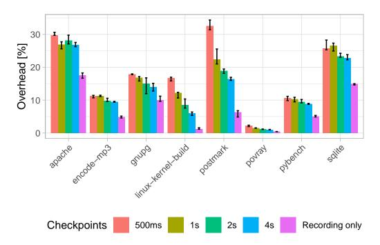
Figure 3.1: Checkpointing can cause a considerable slowdown. Memory-intensive benchmarks such as postmark are particularly affected by the overhead.
