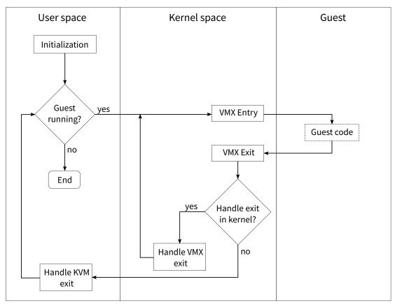
Figure 2.1: Hypervisors can provide a particular environment for guests by handling KVM exits.
