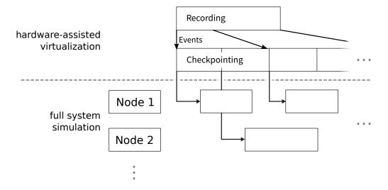
Figure 3.2: Using three stages to remove the checkpointing overhead from the recording. The probe effect caused by the checkpointing is no longer affecting the measurements in the analysis.
