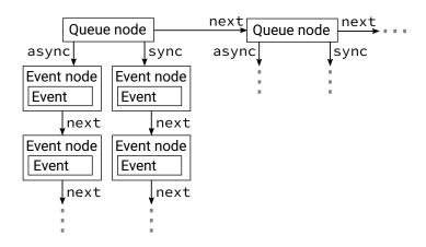
Figure 5.1: The events are transported using a queue, which contains a list for synchronous and asynchronous events. Batches of multiple events are wrapped into a queue node to reduce the run-time cost using atomic instructions to insert new events into the queue.
