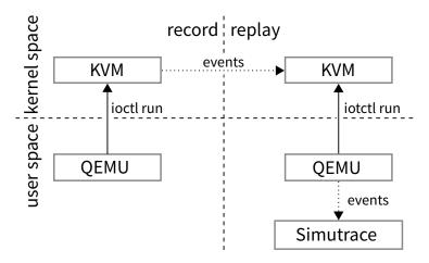
Figure 4.1: The recording is modified to pass any generated events to the replay. Afterwards, the replay engine writes them into Simutrace.
