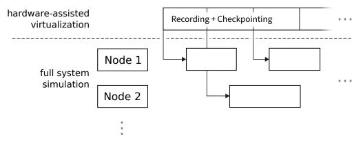
Figure 2.2: The workload is recorded on a hardware-assisted virtual machine and checkpoints are created in regular intervals. The resulting segments are distributed to a pool of worker nodes.
