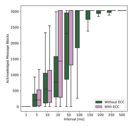
Figure 5.1: Number of Acknowledged Message Blocks Before a Program Crash for Different Bit-Flip Intervals
