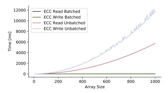
Figure 5.3: Time for Accessing all Elements of an ECC-Protected Array, with and without Batching of ECC calculations
