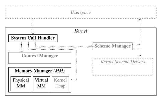
Figure 4.1: Modified Components of the Redox Kernel
