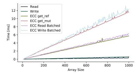
Figure 5.2: Time for accessing all Elements of an Array, with and without ECC Protection
