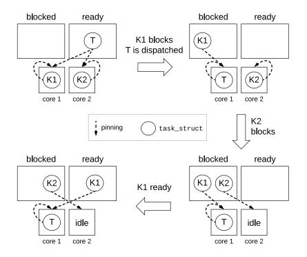
Figure 3.1: The proof-of-concept implementation is not work-conserving. When K1 becomes ready it should be dispatched to C2 immediately. But K1 is pinned to C1 due to the implementation of thread migration.
