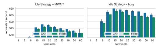
(a) TPC-C throughput. The y-axis is off-set. Error bars represent standard deviation.
