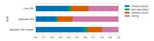
(a) Top-down analysis top-level breakdown. The true frontend-boundedness of MySQL on upstream OSv is only visible when removing spinning in the idle thread, which we did with the mwait configuration. The break-down corresponds to the observations made by Kanev et al. (Section 2.6).
