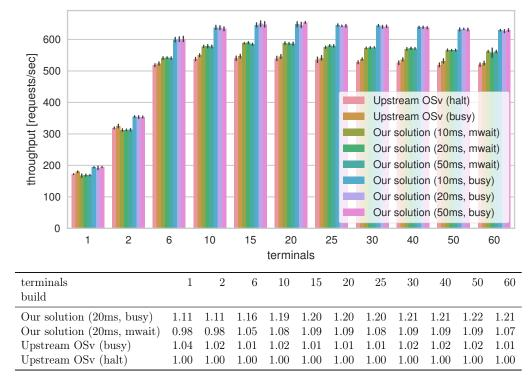
(a) TPC-C throughput and corresponding speedup with upstream OSv as the baseline. Our solution is 22% faster than upstream with busy-waiting 9% faster when using MWAIT in the idle thread. The max\_assignment\_age parameter (left in parentheses) does not significantly affect the performance of our solution.
