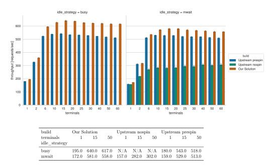
Figure 5.6: TPC-C throughput achieved with fixed core allocation over varying number of terminals. The error bars represent standard deviation over 8 benchmark runs. Our solution increases single-terminal throughput by 8-9% and up to 18% for multi-terminal with busy-waiting. upstream pre-spin is very similar to upstream busy-waiting, whereas upstream nospin is almost 50% slower, showing that upstream pre-spin practically never actually halts the CPU.
