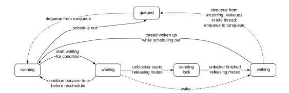
Figure 4.4: Upstream OSv wake-up-related thread state transitions: States *waiting*, *sending\_lock* and *waking* are ambiguous with regard to whether the thread is still scheduling out whether it has fully stopped executing. Dashed lines represent events asynchronous to thread execution, solid lines represent synchronous events.
