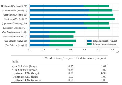
(a) L2 cache misses with 1 and 50 TPC-C terminals. The table below shows the relative amount of code and data misses for 50 terminals with *Upstream OSv (halt)* as a baseline. The 65% reduction of L2 code misses shows the effectiveness of instruction working set spreading.
