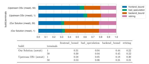
(b) Top-down analysis top-level breakdown at 15 terminals using MWAIT in the idle thread. Our solution shifts 27 percent points from *frontend-bound* to *backend-bound* and *retiring*.
