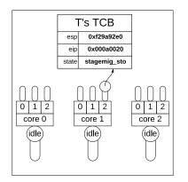
(c) T schedules out. The context switching routine sets its state to stagemig\_sto after T has stopped running on core2.
