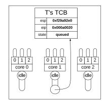
(d) The idle thread on core1 observes T in state stagemig\_sto and admits it to the ready queue.
