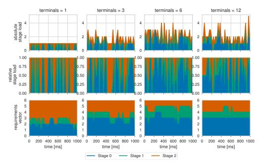
(a) Stage load and resulting requirements vector over time. The exponentiallydecaying average filter smoothens the very spiky stage load profile.
