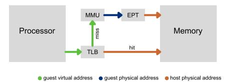
Figure 2.1: On a memory access, the processor forwards the guest virtual address to the TLB for translation. Should the cache not contain a suitable translation, it will trigger a page walk on the MMU and EPT to receive the host physical address necessary to access the memory.
