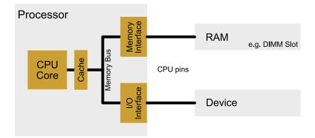
Figure 3.1: Hardware-tracing techniques can only source their information directly from the CPU pins and interfaces inheriting their information from those. They cannot access the CPU core directly to, e.g., obtain the current instruction pointer.
