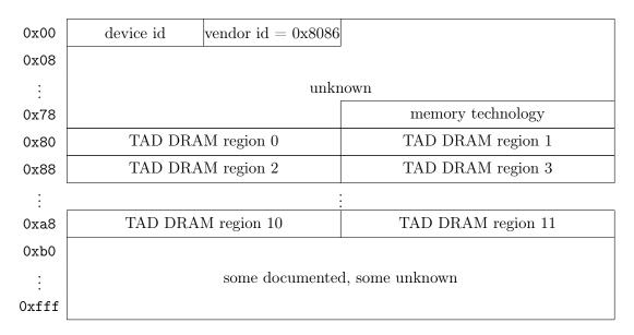
Figure 3: Layout of the integrated memory controller's target address decoder PCI configuration space, device 19, function 0 (13.0). The TAD supports up to 12 different regions. The PCI device id is 0x2fa8 on Haswell and 0x6fa8 on Broadwell-EP. Please refer to the datasheets for documentation of the memory technology register [7, §2.1.2, 6, §2.1.2].
