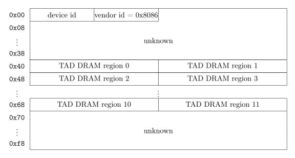
Figure 2: Layout of the home agent's target address decoder PCI configuration space, device 18, function 0 (12.0). The TAD supports up to 12 different regions. The PCI device id is 0x2fa0 on Haswell and 0x6fa0 on Broadwell-EP.
