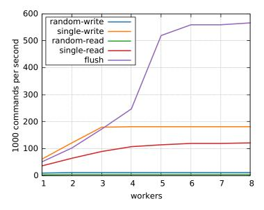
Figure 5.3: NVMe command rate on Sandy Bridge with our modified Kernel.
