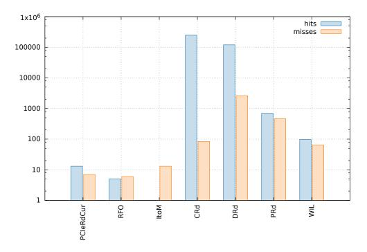
Figure 5.4: Performance counter results of running the counters for 5 s without any load on a logarithmic scale.
