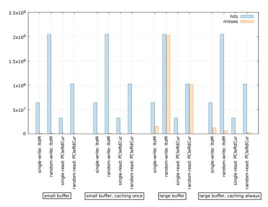
Figure 5.7: Comparison of PCM event counts with different buffer sizes and caching modes in nvme-memload. Only events including transferred data blocks are shown.
