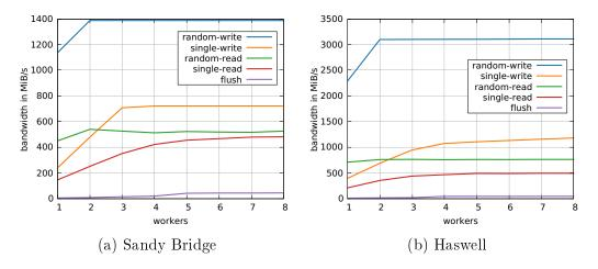
Figure 5.1: DMA bandwidth used by nvme-memload with different amounts of worker threads sending NVMe commands.
