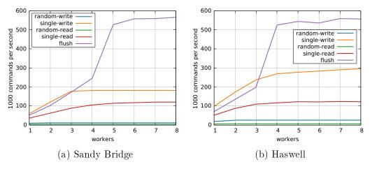
Figure 5.2: NVMe command rate of nvme-memload with different amounts of worker threads.
