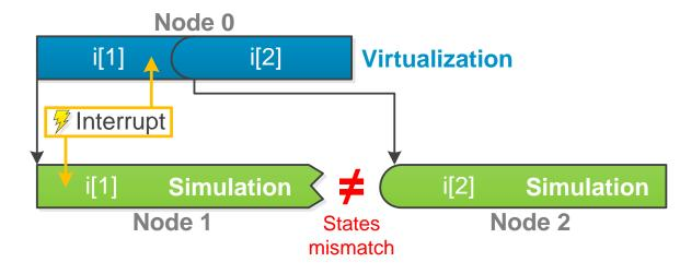
Devices work asynchronous to CPU
