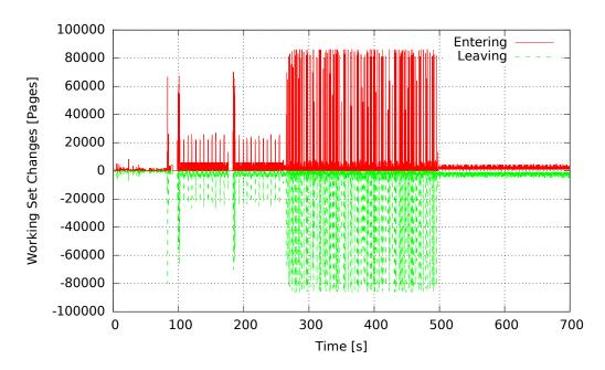
Figure 1: The write working set changes of a VM running SPEC.433.milc (1024 MiB memory).
