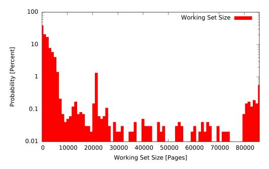
Figure 2: The distribution of write working set sizes of SPEC.433.milc.
