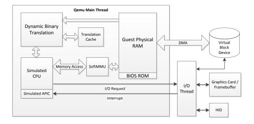
Figure 2.5: The organization of QEMU. It consists of two threads, one for CPU simulation and one for device emulation. The interaction is similar to a real system, but interrupt delivery can be postponed.
