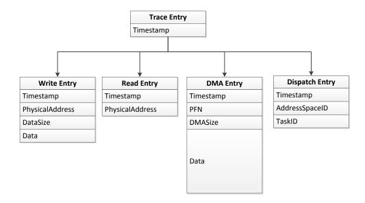
Figure 5.8: Typical trace entries, as actually used for the data acquisition. Every entry consists of a timestamp to correlate it with other data streams.
