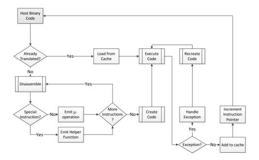
Figure 2.4: Dynamic binary translation and the typical work-flow of disassembling, translation, and execution to correspond to the guest ISA. The binary translator must recreate a *code block*, if an exception, e.g., a page fault has occurred. A successfully executed block is added to a cache to speed up re-execution.
