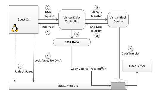
Figure 5.4: The typical DMA processing for storage devices in QEMU intercepted by our hook.
