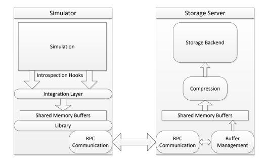
Figure 5.6: The different abstraction layers, which provide a simple integration of the storage server into various simulators. All interfaces are exposed through a small library.
