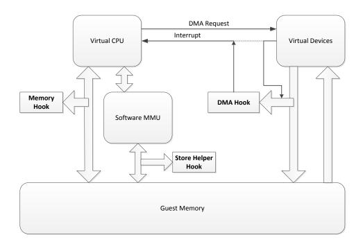
Figure 5.1: Overview over different memory hooks, as necessary to intercept main memory operations in QEMU. The memory hook is invoked most frequently.
