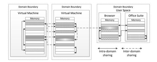
Figure 2.2: The figure shows two VMs (two semantic domains), and native applications, a domain of its own. Pages can be shared within the same domain (*intra-domain*) and across domain boundaries (*inter-domain*).
