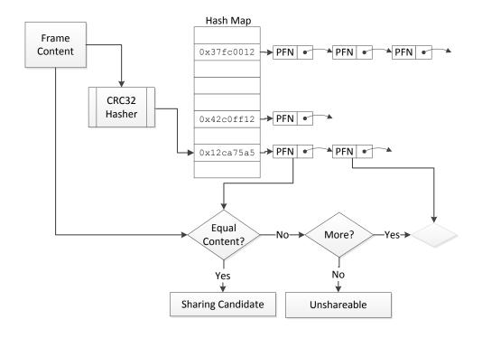
Figure 5.12: The process from page frame content to the detection of a sharing opportunities. The chained hash map speeds up detection and avoids false positives.
