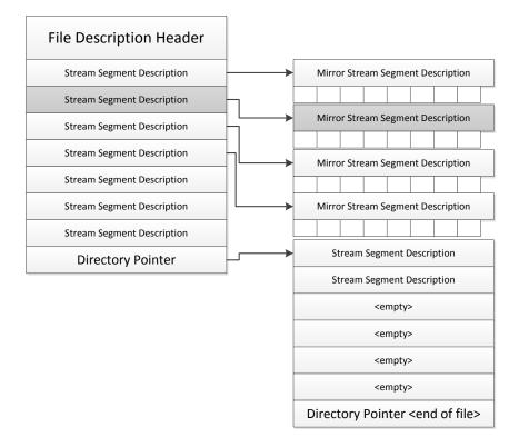
Figure 5.7: The layout of a trace file. It consists of a file header for metadata, directories, for fast stream access, and stream segments, for actual data storage.
