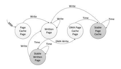
Figure 6.1: A simplified HMM for the Linux page cache. It shows a sub-set of possible transitions. All unmap transitions are omitted.
