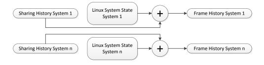
Figure 4.5: The recovered OS system state is fused with the information from the memory reconstruction, to form a compact page frame history.
