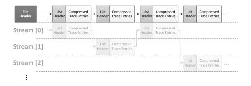
Figure 4.2: The previous trace file format stores a linked list of variablesized trace-lists. Each list comprises a header and compressed trace entries. The lists are tagged to associate them with the corresponding streams [41].
