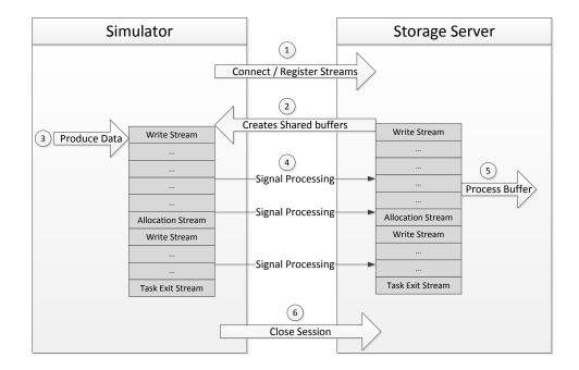
Figure 5.10: A typical service scenario: A simulator connects to an instance of a storage server and registers its streams. In return a shared buffer is created and the simulation can produce and commit trace data.
