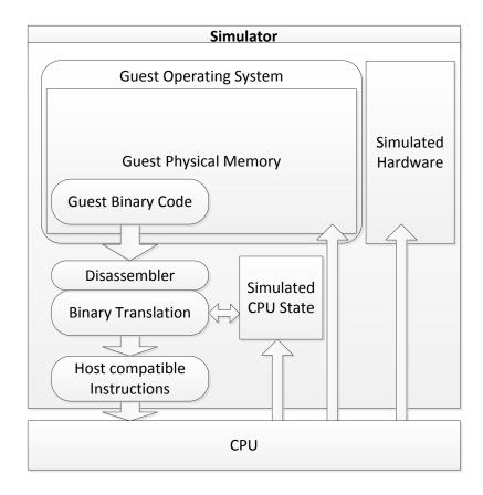
Figure 2.3: The general work-flow of a simulator using *binary translation*. The guest code is disassembled, translated, typically instrumented, and executed on the hosting platform. All memory accesses have been modified to point into the guest assigned memory regions.
