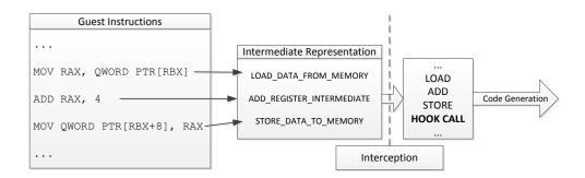
Figure 5.2: The binary translator disassembles guest instructions and maps them to a compact intermediate representation. Every intermediate load or store instruction is extended with a memory hook callback.
