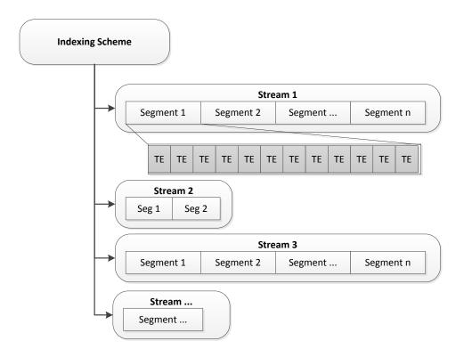
Figure 4.3: A trace store consists of streams. Each stream consists of segments, which contain fixed-size trace entries. A fast indexing scheme avoids cumbersome data discovery on trace loading.
