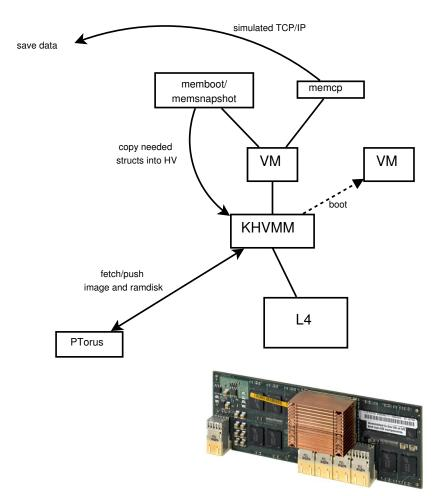
Figure 3.2: Illustration how data is saved and loaded to deploy VMs. The VM copies needed data into the hypervisor which then issues the data transfer and the booting procedure
