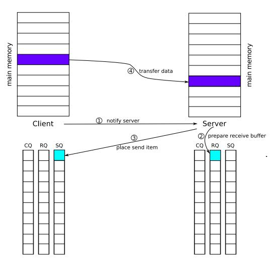
Figure 3.3: RDMA data transfer from the client to the server.
